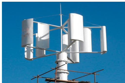
Figure 2. Vertical-axis wind turbine. Reprinted from Li [23] with permission under the terms of the Creative Commons Attribution License ( http://creativecommons.org/licenses/by/3.0 )
