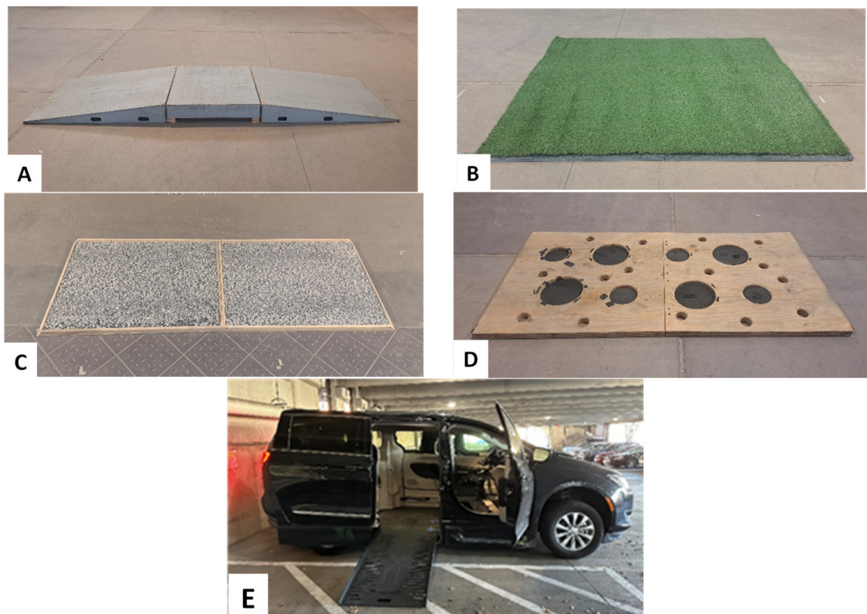
Figure 3. Wheelchair test course. (A) Curb cut, (B) Grass, (C) Gravel, (D) Potholes 1" depth, (E) Accessible vehicle.
