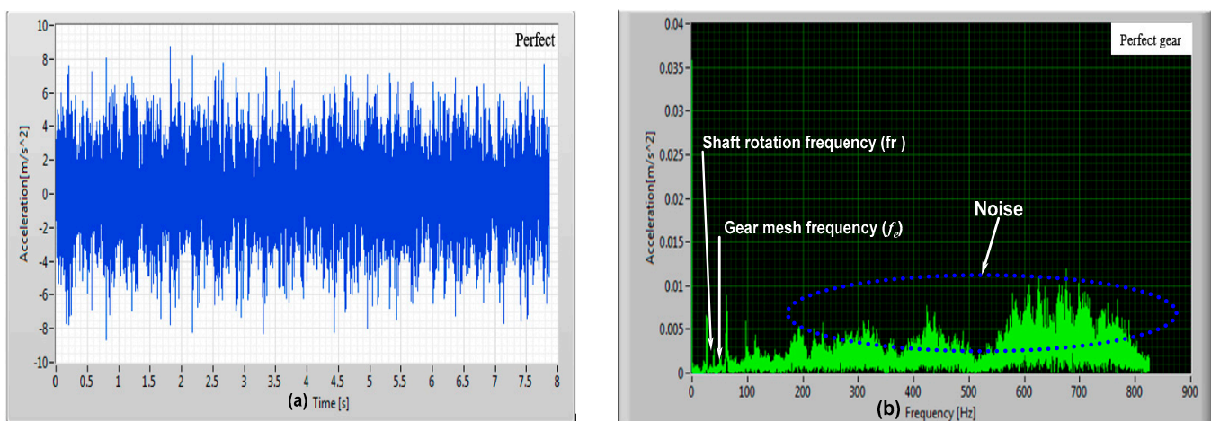
Figure 14. Responses of a healthy gear: (a) Time-domain (b) Spectrum (FFT).
