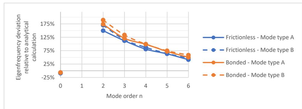
**Figure 8.** Effect of stator frame with bonded and frictionless contact between core and double-dovetail bars.
