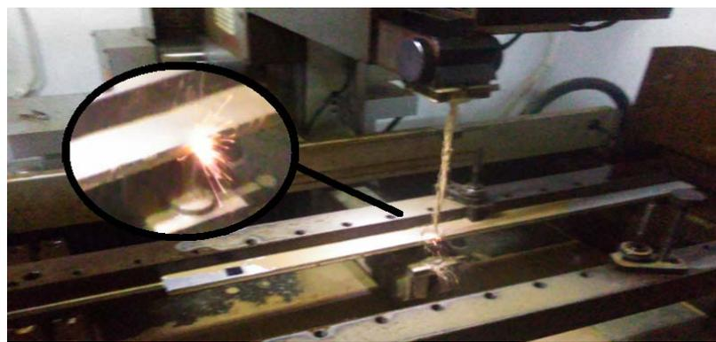
Figure 10. Crack Creation with a wire-cut electro-erosion machine.
