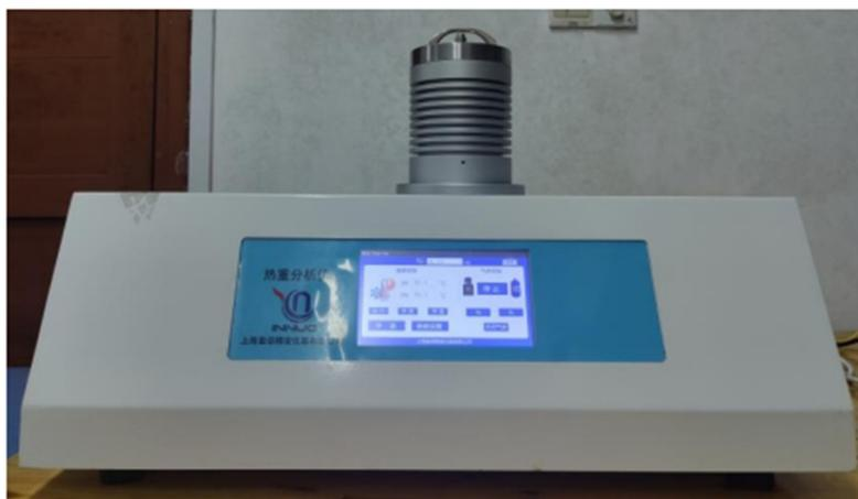
Figure 1. TGA-1150 thermogravimetric analyzer.
