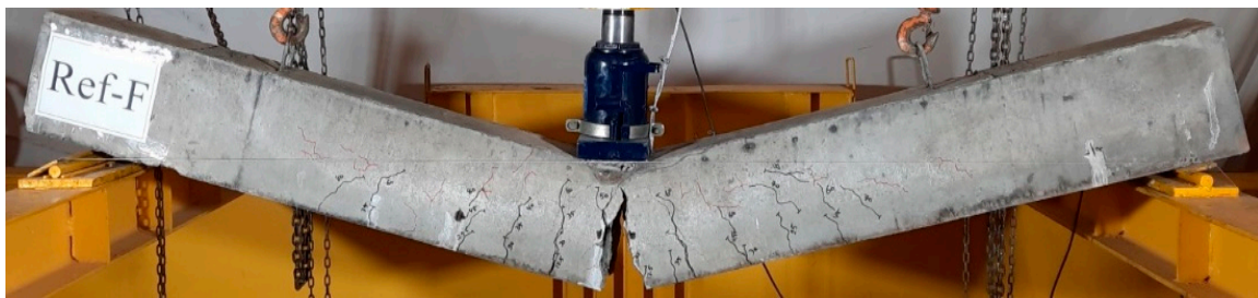
Figure 11. Crack patterns and failure mode of beam Ref-F.
