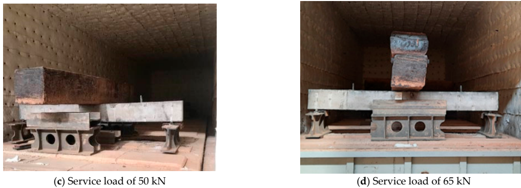
Figure 7. The service load at the mid-span of each beam during fire loading.
