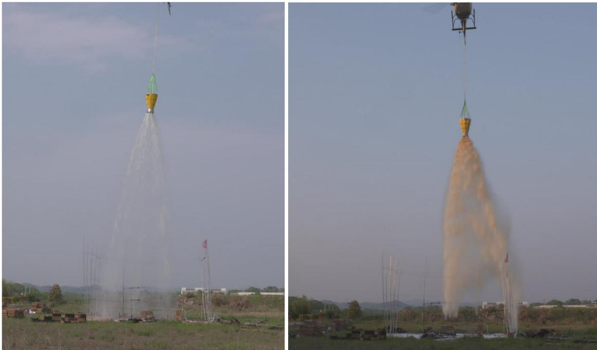
**Figure 8.** Helicopter high-altitude spraying of flame retardants. **(Left):** gel fire-extinguishing agent; **(Right):** class AB fire-extinguishing agent.
