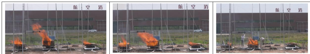
**Figure 9.** Combustion conditions of the fire scenes in the model without spraying flame retardants onto the wood crib. First subgraph: 180 s; second subgraph: 600 s; third subgraph: 870 s.
