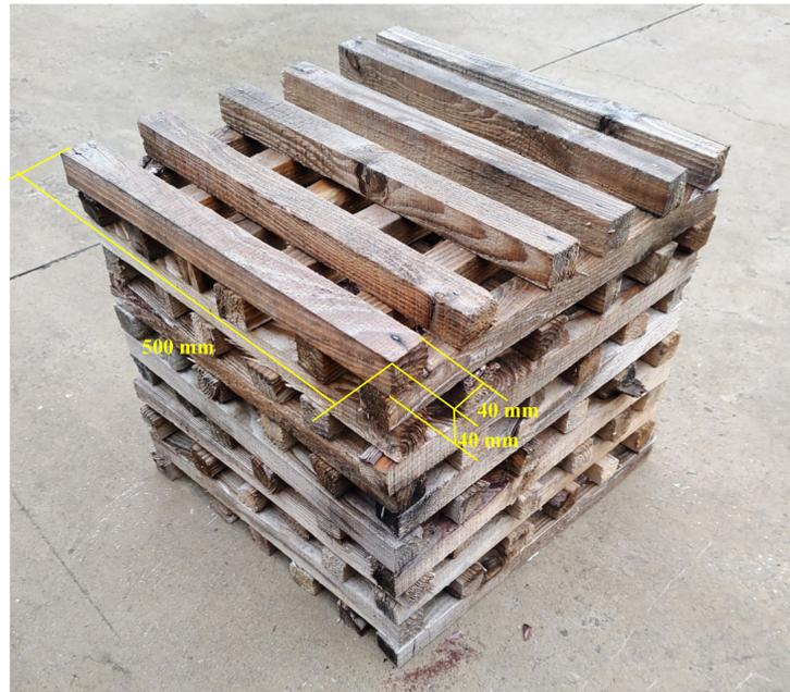
**Figure 2.** Photograph showing the construction of the 12-layer wood cribs.
