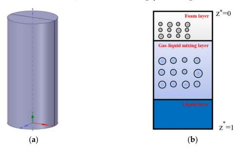
**Figure 1.** Modelling setup. The aerated mixture can be divided into three layers: the foam layer, the gas-liquid mixing layer, and the liquid layer. (a) Three-Dimensional Model. (b) *xy*-Plane Slice.
