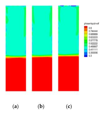
**Figure 8.** Distribution of the liquid volume fraction of *xy*-plane slice during the separation process at 60 s, where the surface tensions are  $\sigma = 0.04$  (a),  $\sigma = 0.055$  (b),  $\sigma = 0.07$  (c), respectively.
