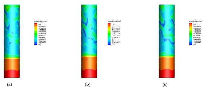
**Figure 4.** Distribution of the gas-liquid-foam during the separation process at 30 s, where the grid numbers are 65,500 (a), 126,000 (b), and 183,700 (c), respectively.
