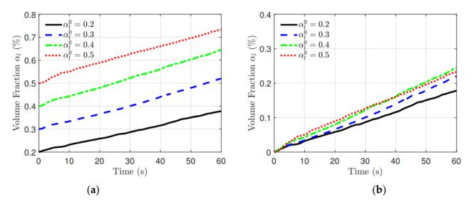
**Figure 14.** Time history of the volume fraction of the liquid, where the initial volume fractions of the liquid are different, namely,  $\alpha_l^0 = 0.2, 0.3, 0.4$ , and 0.5. (a) Volume fraction of the liquid. (b) Initial volume fraction is subtracted.
