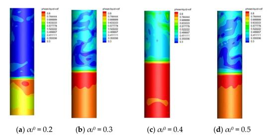
**Figure 13.** Distribution of the liquid volume fraction at t = 50 s,  $\alpha_l^0 = 0.2, 0.3, 0.4$ , and 0.5.
