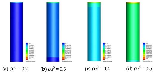
**Figure 12.** Distribution of the liquid volume fraction at t = 5 s, where  $\alpha_t^0 = 0.2, 0.3, 0.4$ , and 0.5.
