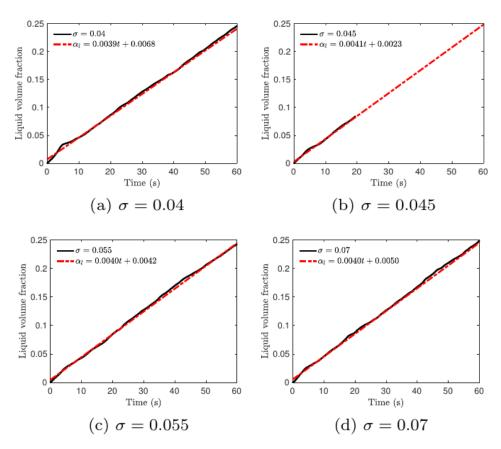
**Figure 10.** Curves of the liquid volume fraction with the time, together with the linear fitting results, where the surface tensions are different.
