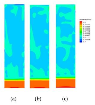
**Figure 7.** Distribution of the liquid volume fraction of *xy*-plane slice during the separation process at 30 s, where the surface tensions are  $\sigma = 0.04$  (**a**),  $\sigma = 0.055$  (**b**),  $\sigma = 0.07$  (**c**), respectively.
