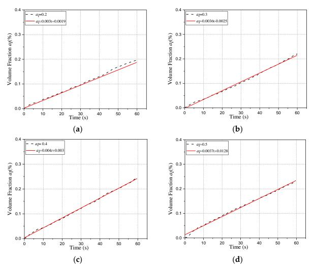
**Figure 15.** Curves of the liquid volume fraction with the time, together with the linear fitting results. (a)  $\alpha_l^0 = 0.2$ . (b)  $\alpha_l^0 = 0.3$ . (c)  $\alpha_l^0 = 0.4$ . (d)  $\alpha_l^0 = 0.5$ .
