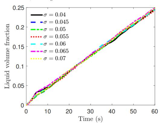
**Figure 6.** Evolution of the liquid volume fraction with time, where different surface tensions are adopted.
