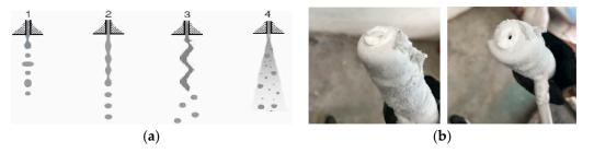
**Figure 6.** Liquid nitrogen ejection from solid conical spray nozzles: (**a**) Different patterns for atomization of solid nozzles; (**b**) Frosting phenomenon at the outlet of nozzles.
