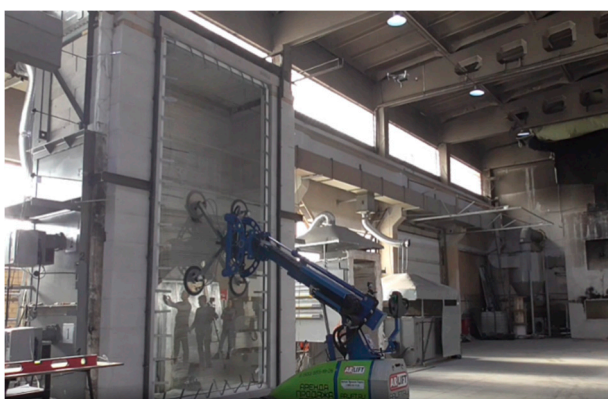
Figure 4. Installation of a monolithic single-layer glass panel in the furnace opening. Photo by the authors.
