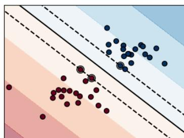
**Figure 1.** An SVM example. Here, the filled circles show the data points, the solid line represents the decision boundary, and the dashed lines represent the support vectors [30].
