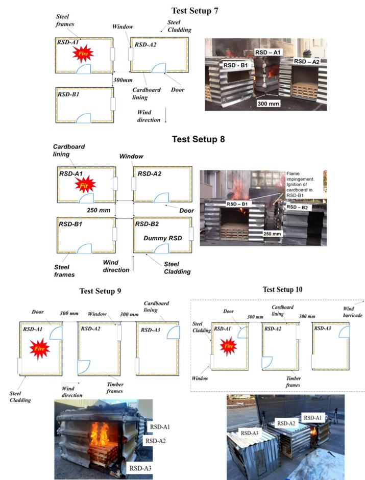
Figure 8. Tests 7 to 10 showing layouts and images during testing.
