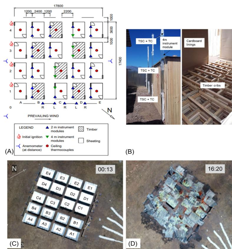
**Figure 3.** Full-scale fire test on 20 informal dwellings. (A) Experiment layout, (B) instrumentation and fuel load arrangement, (C) aerial image of fire experiment soon after ignition, (D) image of fire experiment at 16 min 20 s [10].
