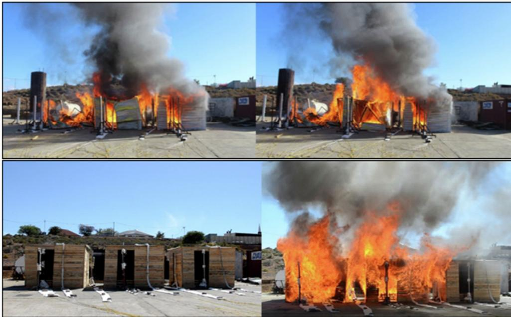
**Figure 2.** Fire spread between multiple full-scale informal dwellings. (Top) Steel-clad dwellings, (bottom) wooden-clad dwelling [7].
