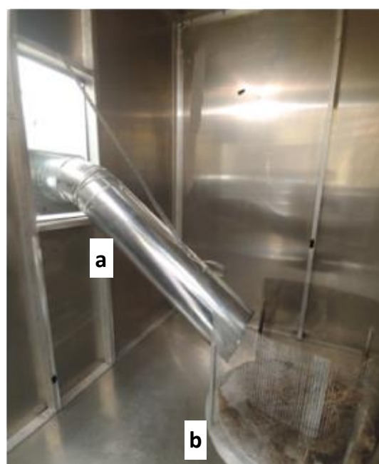
Figure S1. DRI combustion chamber with (a) fuel-delivery system and (b) burning platform (round ceramic disc on the bottom right).
