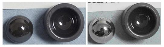
Figure 18. Silicon nitride acetabular cup and femur head before and after 1 million cycles [25].
