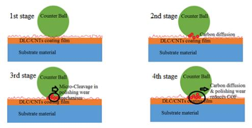
Figure 10. Representation of the different stages of wear in DLC materials [76].
