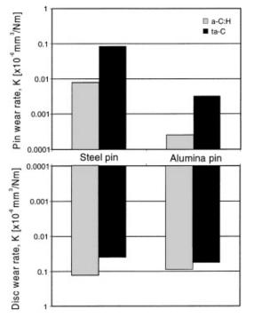
Figure 11. Wear rates of pin and disc in pin on disc friction test performed on a-C and a-C:H [77].
