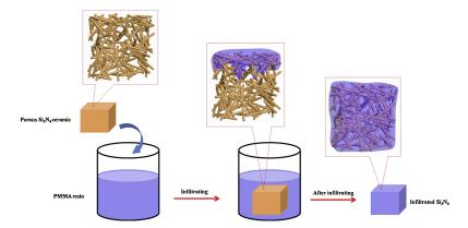
Figure 15. Process of silicon nitride matrix infiltration [86].
