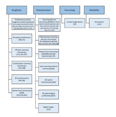
Figure 15. Methods/equipment used in publications for the evaluation of the surface properties.
