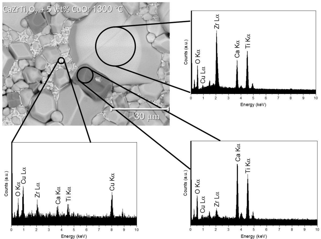
**Figure 5.** SEM/EDS analysis of CaZrTi<sub>2</sub>O<sub>7</sub> + 5 wt.% CuO sintered at 1300 °C.
