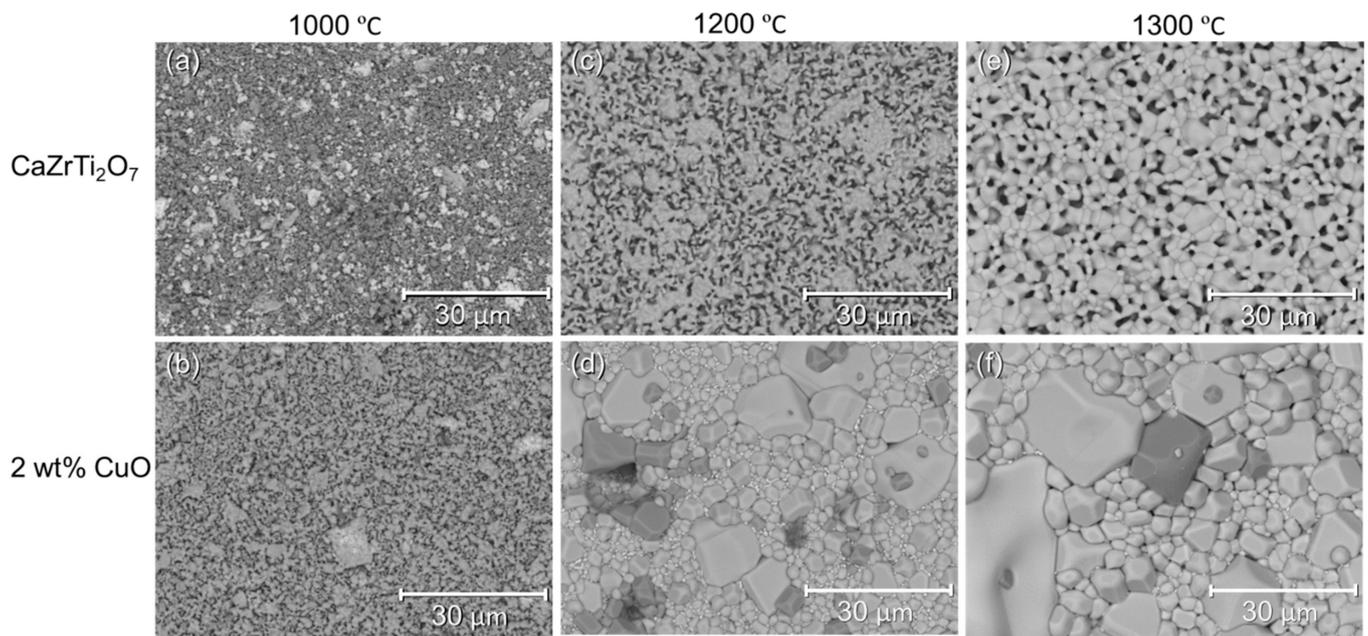
**Figure 4.** Scanning electron micrographs of (a) undoped CaZrTi<sub>2</sub>O<sub>7</sub> sintered at 1000 °C; (b) 2 wt.% CuO sintered at 1000 °C; (c) undoped CaZrTi<sub>2</sub>O<sub>7</sub> sintered at 1200 °C; (d) 2 wt.% CuO sintered at 1200 °C; (e) undoped CaZrTi<sub>2</sub>O<sub>7</sub> sintered at 1300 °C; (f) 2 wt.% CuO sintered at 1300 °C.
