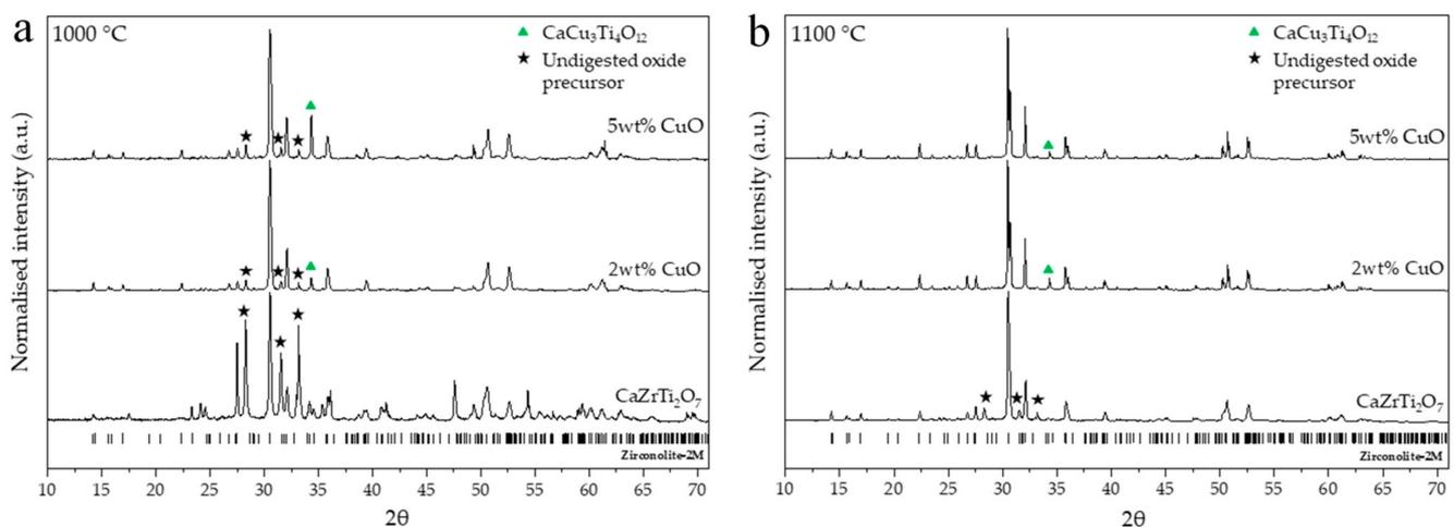
**Figure 1.** Powder X-ray diffraction data obtained for compositions synthesised at (a) 1000 °C and (b) 1100 °C. CaCu<sub>3</sub>Ti<sub>4</sub>O<sub>12</sub> characteristic reflections are highlighted with green triangles and precursor phase reflections are highlighted with black stars.
