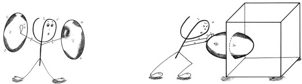
Figure 8. Adjusted quasi-phi-functions for appropriate geometries are used for describing non-overlapping of components with minimal allowable distances (left) and phi-functions are applied for containment of components in the cuboidal container (right).
