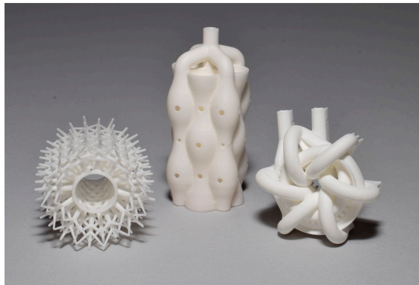
Figure 22. Ceramic heat sinks (left and right) and static mixer (centered) manufactured at Fraunhofer IKTS via CerAM VPP with the CeraFab 7500 device and LithaLox 350 suspension of Lithoz.
