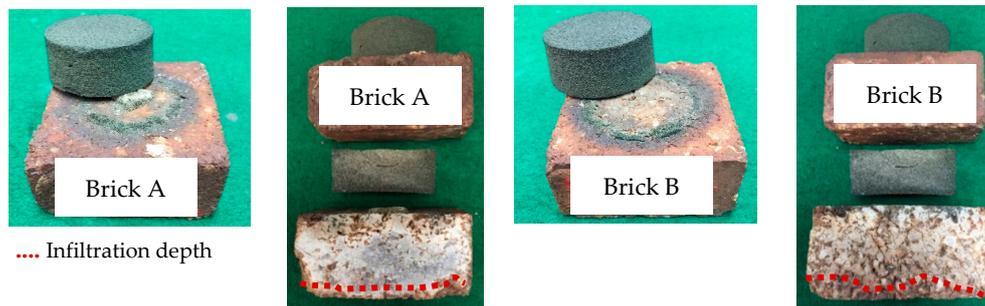
**Figure 5.** Visual aspect and cross section of the bricks A and B after 3 cycles of contact coating test using modified cement raw meal.
