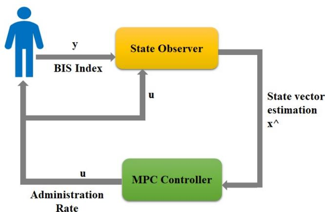
**Figure 9.** NMPC closed-loop structure in anaesthesia.
