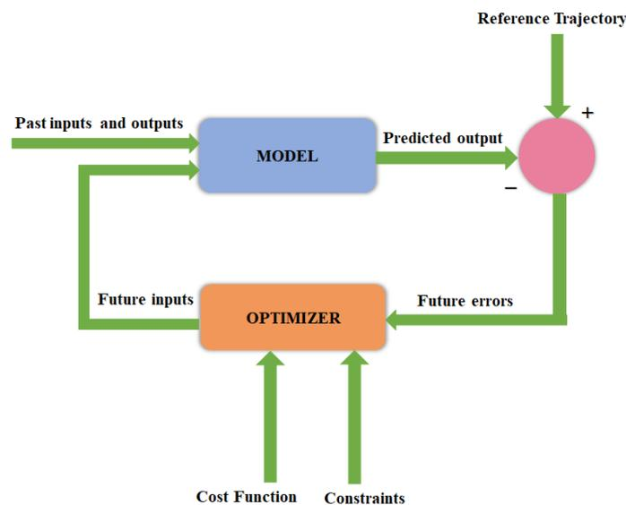
**Figure 3.** Basic structure of MPC.
