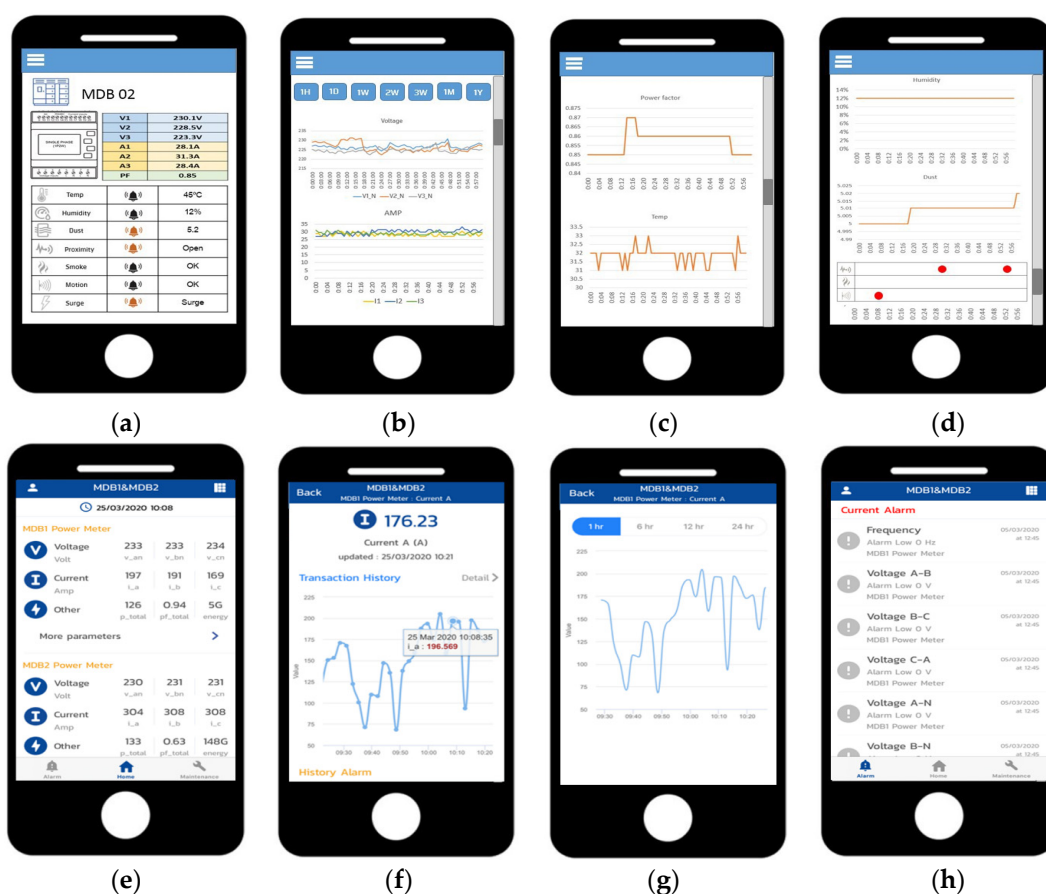
Figure 5. Display of the results via a smartphone device to control an electric switchboard, consisting of (a) various system notification settings, (b) the amount of electricity consumption, (c) the current electric power and temperature, (d) the amount of humidity inside the switchboard, (e) power quality and related parameters, (f) power quality and parameters in graph model, (g) graphs reporting the past 24 h of electricity consumption, and (h) electrical fault warning area in the switchboard.
