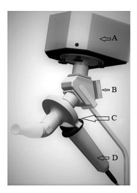
**Figure 1.** Impulse oscillometry assembly consisting of sound emitter (A), screen flap (B), Y-adapter with a mouthpiece (C), pneumotach (D)
