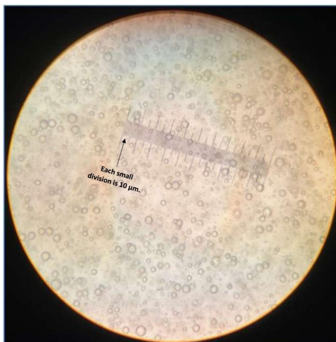
Figure 17. Typical photomicrograph of O/W emulsion stabilized and thickened by nanocrystalline cellulose.
