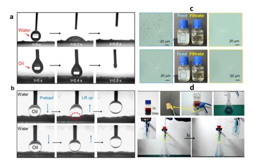
**Figure 11.** (a) Rapid water and oil spread over the membrane as shown by high-speed photography. (b) Dynamic images demonstrating the oil repellency and oil adhesion of CSNFMs and BC- CSNFMs while submerged in oil. (c) Digital photographs for silicone-in-water SFE (up) and SSE (down) before and after separation. (d) Demonstration of separation of immiscible oil-water mixtures. [140]. Reprinted with permission from Ref. [140] Copyright 2022 Elsevier B.V. All rights reserved.
