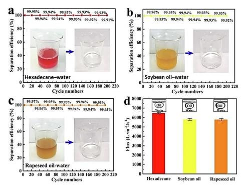
**Figure 10.** Separation efficiencies of CuO@PAA membrane for various oil–water combinations (**a**–**c**) and water penetration fluxes (**d**). Insets 10a, b, and c show oil–water combinations and filtered water; 5d shows hexadecane, soybean oil, and rapeseed oil on CuO@PAA membrane in water [139]. Reprinted with permission from Ref. [139]. Copyright © 2023 Elsevier B.V. All rights reserved.
