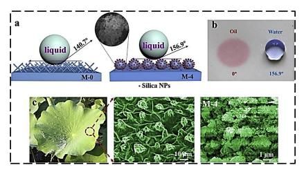
**Figure 6.** (a) Diagrams illustrate the effect of bottom surface structure of M-0 and M-4 on the hydrophobic; (b) Photograph of pure water and oil droplets on the M-4 bottom surface; (c) Optical photograph and SEM image of lotus leaf [119]. Reprinted with permission from Ref. [119]. Copyright 2019 Elsevier B.V. All rights reserved.
