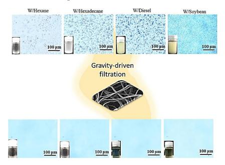
**Figure 7.** Optical micrographs of the feed emulsions (**top part**) and permeates (**bottom part**) using PMMA/60PDMS nanofibrous membrane under the sole influence of gravity [121]. Reprinted with permission from Ref. [121]. Copyright © 2023 Elsevier B.V. All rights reserved.
