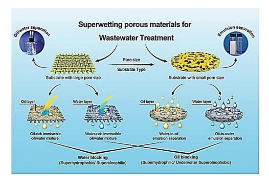
**Figure 3.** Design of the superwetting porous materials and the mechanism of oil/water separation or emulsion separation [100]. Reprinted with permission from Ref. [100] Copyright © 2023 WILEY-VCH Verlag GmbH & Co. KGaA, Weinheim, Germany.
