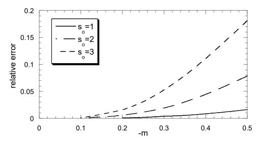
**Figure 1.** Relative error of the method of moment in computation of  $M_1$  (in time such that the exact value of  $M_1$  is 0.1) versus exponent m for three values of the initial dispersity  $s_0$ .
