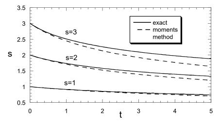
**Figure 2.** Exact and computed results with the method of moments dispersities versus dimensionless time for three values of the initial dispersity s<sub>0</sub>.
