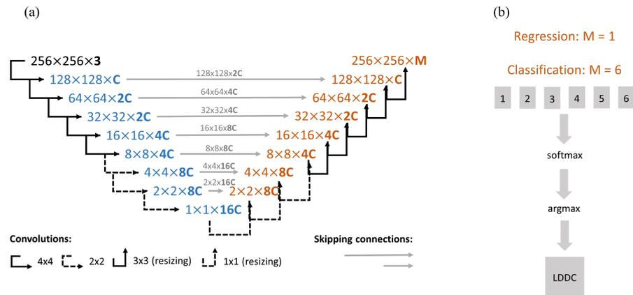
**Figure 5.** (a) Architecture of the CNN; and (b) outputs of the CNN depending on the regression or classification task.
