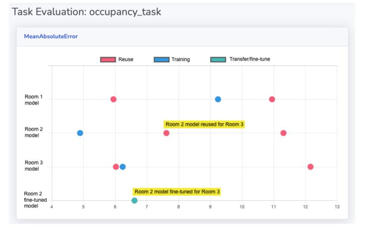
**Figure 8.** Snapshot of inter-space learning prototype for evaluation of occupancy prediction models. On the y-axis the available models for fulfilling the occupancy prediction are shown and the x-axis represents the Mean Absolute Error (MAE) for comparing the performance of those models.
