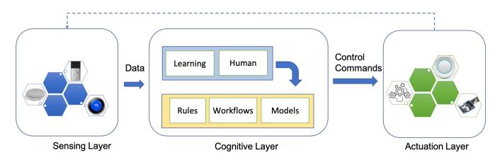
Figure 1. Three-layer model of an Internet of Things (IoT)-based system including sensing, context, and actuation layers.
