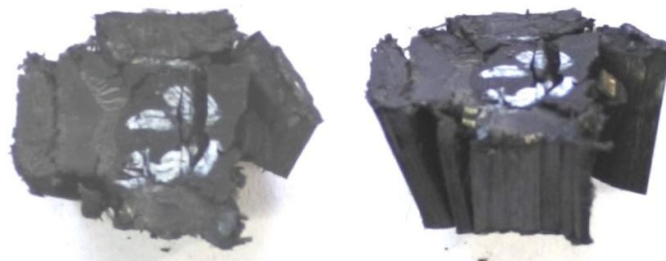
Figure 14. Failure patterns of the specimens of the fiber direction tests.
