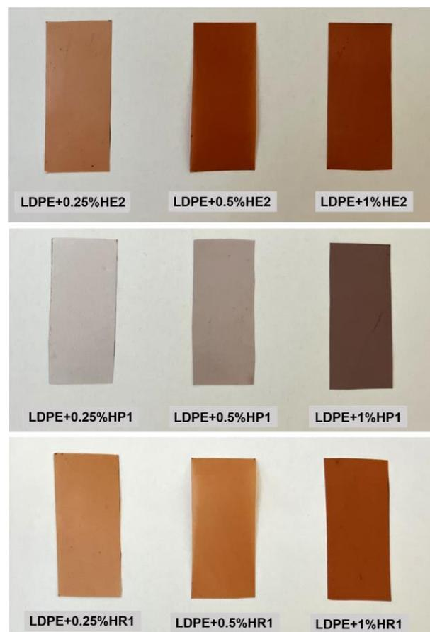
**Figure 1.** Photographs of prepared LDPE/hematite composites.
