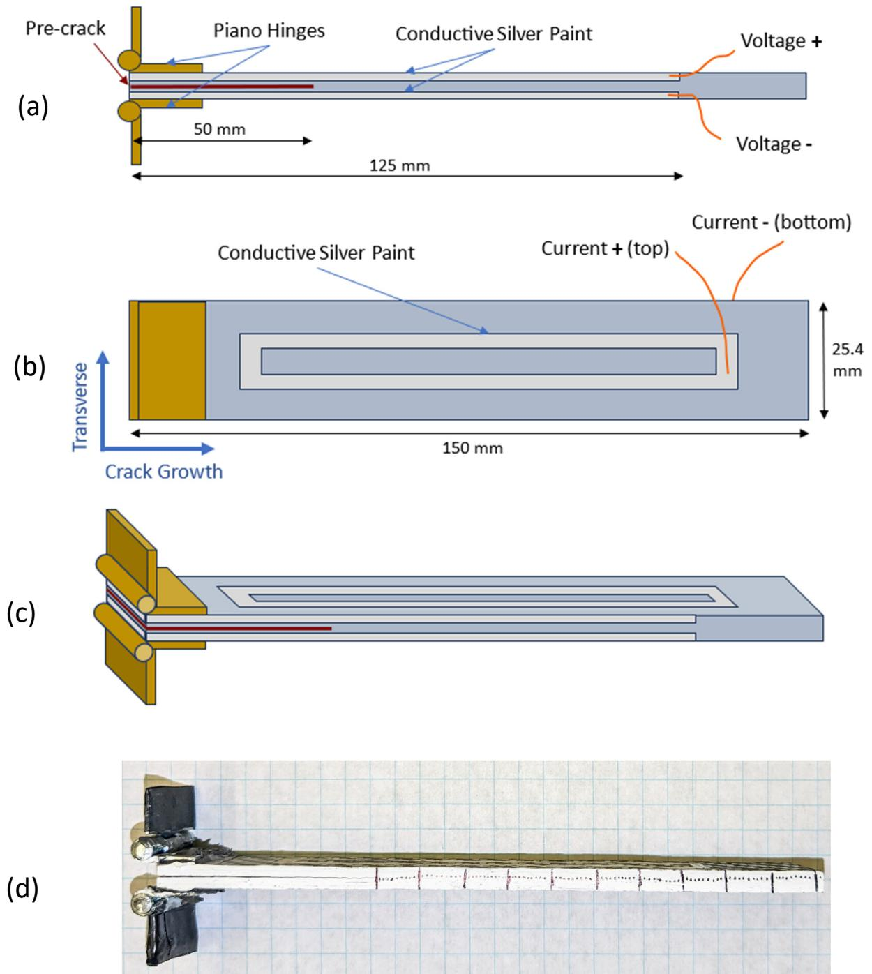
**Figure 3.** Diagram of DCB specimen configuration, with (a) showing the side view with voltage probes, (b) showing the top view with current probes, (c) showing a 3D view of the specimen where the voltage probes go around the crack faces, and (d) showing a side view of the actual test specimen.
