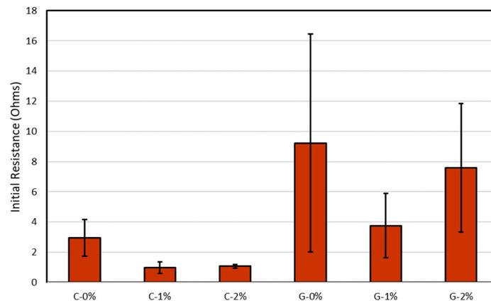
**Figure 8.** Initial resistance for each composite configuration.
