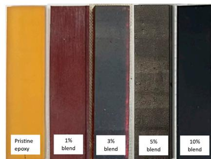
**Figure 1.** Image of bar shape (ASTM D790) of re-blended epoxy with different REP compositions.
