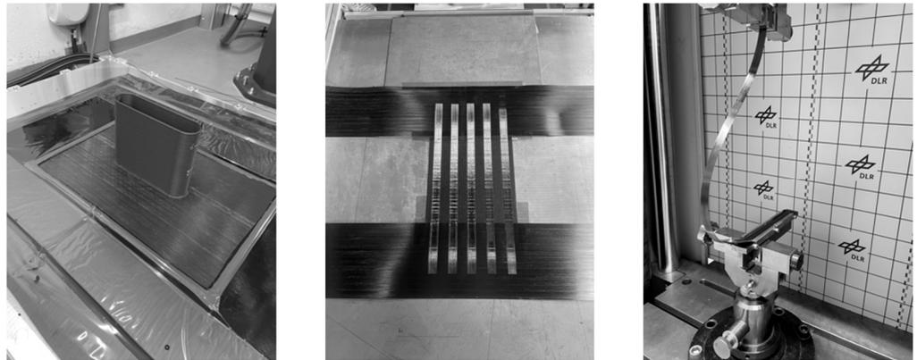
**Figure 4.** Preparation of Peel Specimens [1]. 3D printing of Substrates (left), AFP on substrate (middle), Testing of specimens (right).
