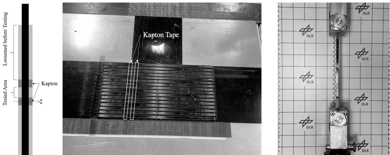
**Figure 3.** Preparation of DLS Specimens.
