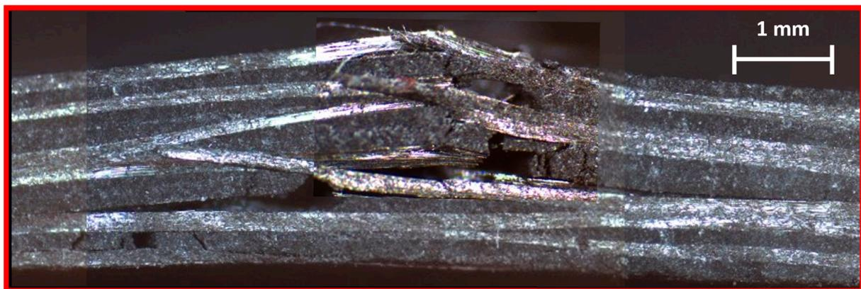
**Figure 7.** Fractured longitudinal section of a tensile specimen manufactured by laying-up plies of  $380 \text{ g/m}^2$ .
