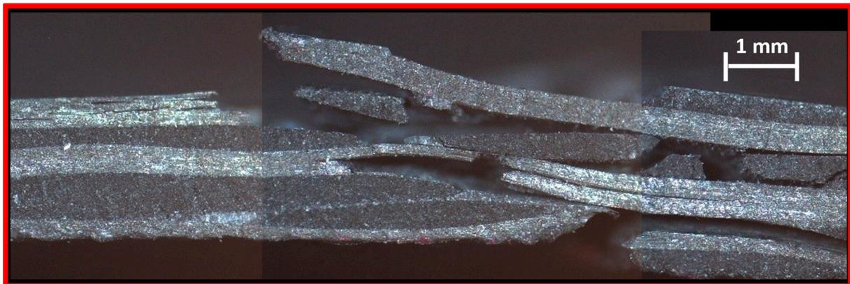
**Figure 9.** Fractured longitudinal section of the tensile specimen manufactured by laying-up plies of 800 g/m<sup>2</sup>.
