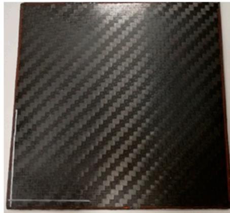
**Figure 1.** A flat laminate in CFRP produced by hand lay-up process, after curing.
