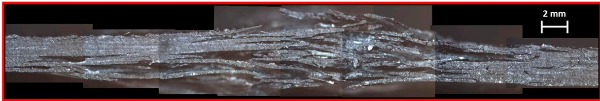
**Figure 10.** Fractured longitudinal section of the in-shear specimen in composite laminate manufactured by laying-up plies of  $380 \text{ g/m}^2$ .
