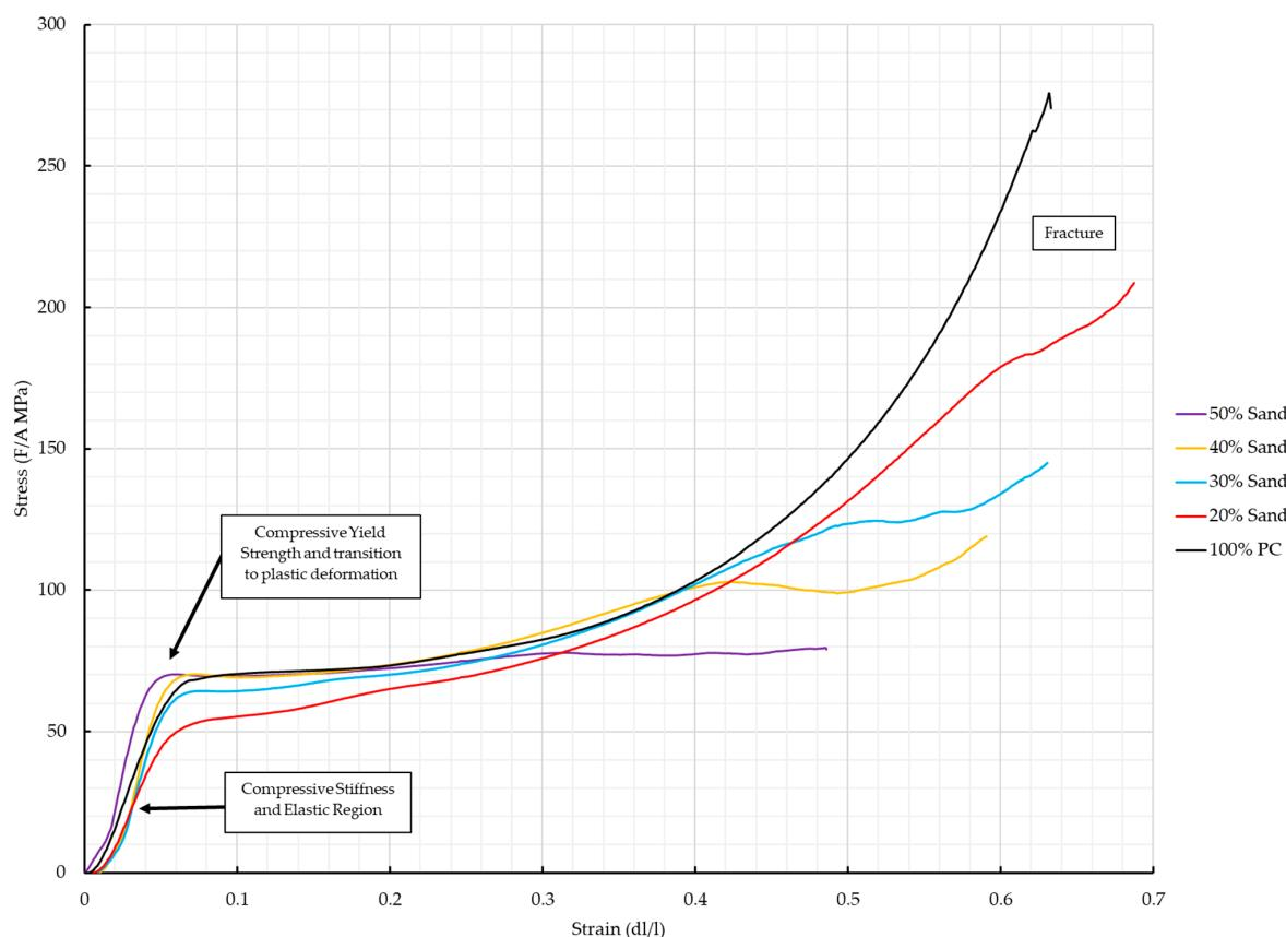
**Figure 8.** Stress vs. strain across a range of sand/PC compositions by weight compared to the optimal 100% PC control. The datasets shown are representative samples of the different compositions.
