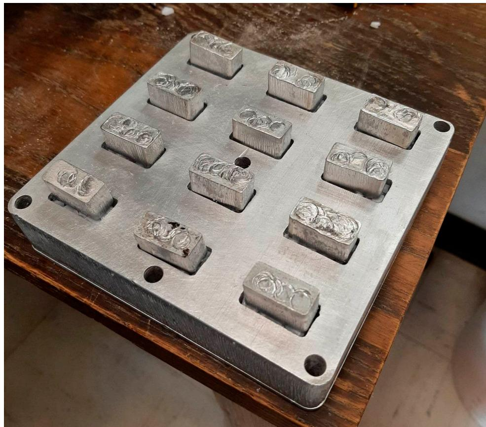
**Figure 4.** Loaded mold before compression.
