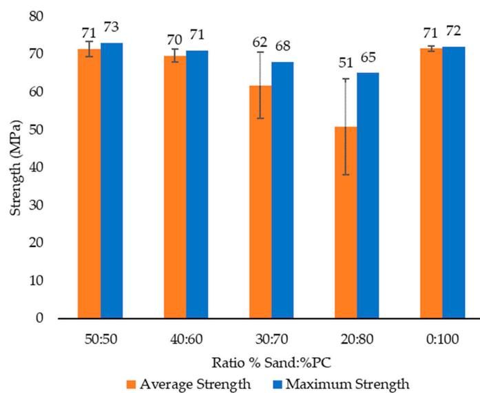
**Figure 9.** Summary of the impact of sand % in the sand/PC composite on maximum strength and average strength (MPa).
