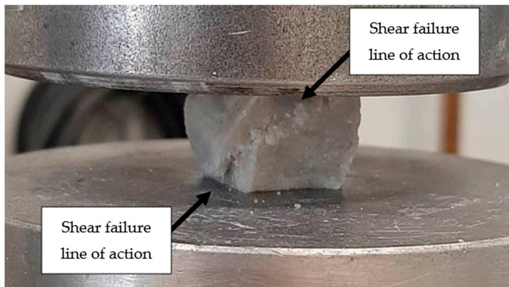
**Figure 11.** Shear failure of the 50% sand sample during compression testing.
