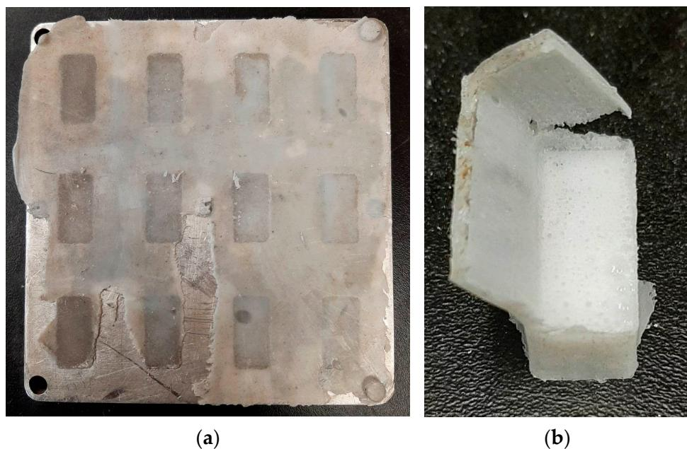
**Figure 6.** (a) Released mold with visible flash. Mold was filled with 50% sand on the left and 20% sand on the right. (b) The 100% PC sample example immediately following part ejection and prior to cleanup.
