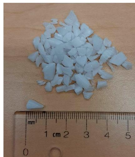
**Figure 1.** Waste PC regrind used to produce all samples.
