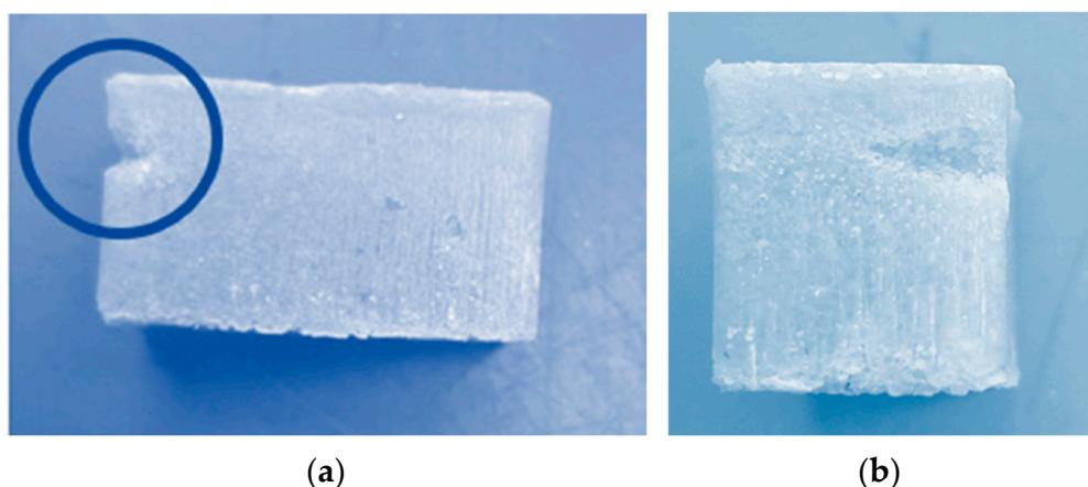
**Figure 12.** Surface defects (circled) caused by plastic sand inhomogeneity during mixing. (a) The 40% sand sample front view, (b) the 40% sand sample side view.
