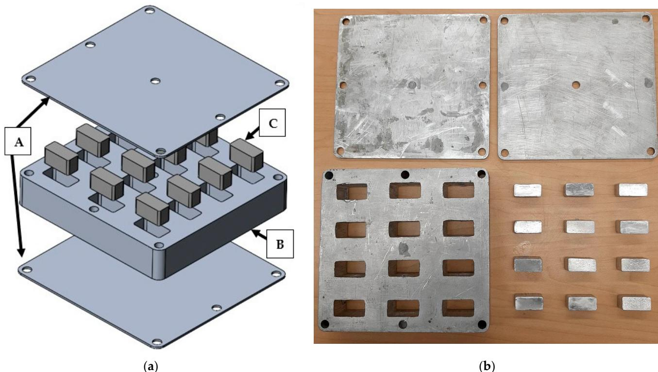
**Figure 2.** Laser-cut aluminum mold components and alignment orientation. (a) 3-D render and (b) physical components of (A) Mold Lid X2, (B) ASTM D695 Pocket Mold, (C) Mold Plug X12.
