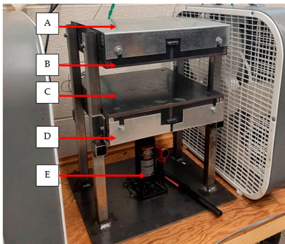
**Figure 3.** Open-source scientific hot press used for manufacturing all samples. (A) Fixed upper plate insulated subassembly and heater enclosure. (B) Fixed upper pressing plate work surface. (C) Adjustable lower pressing plate work surface. (D) Adjustable lower plate insulated subassembly and heater enclosure. (E) A 4-ton bottle jack for vertical actuation.
