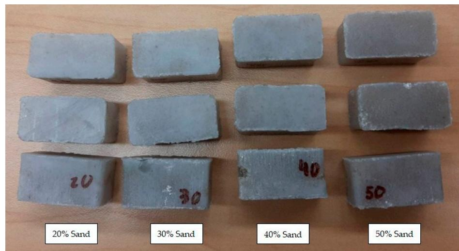
**Figure 7.** Plastic sand bricks matrix of samples. Columns are identified from left to right as 20%, 30%, 40%, and 50% sand-to-plastic ratios by weight.
