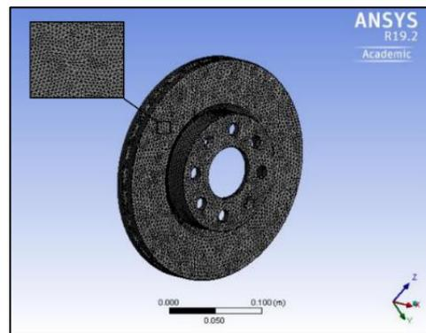
Figure 4. Meshed brake disc.
