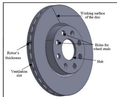
Figure 3. 3D view of brake disc.
