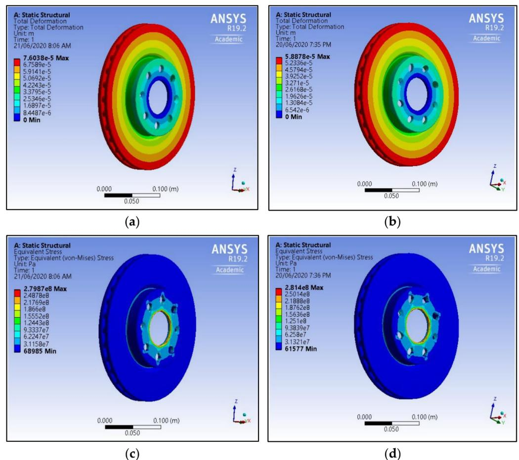
**Figure 6.** Structural analysis of Al/SiC/Gr- and cast-iron-based brake rotors. (a) Deformation—Al/SiC/Gr, (b) Deformation—cast iron, (c) Equivalent stress—Al/SiC/Gr, and (d) Equivalent stress—cast iron.
