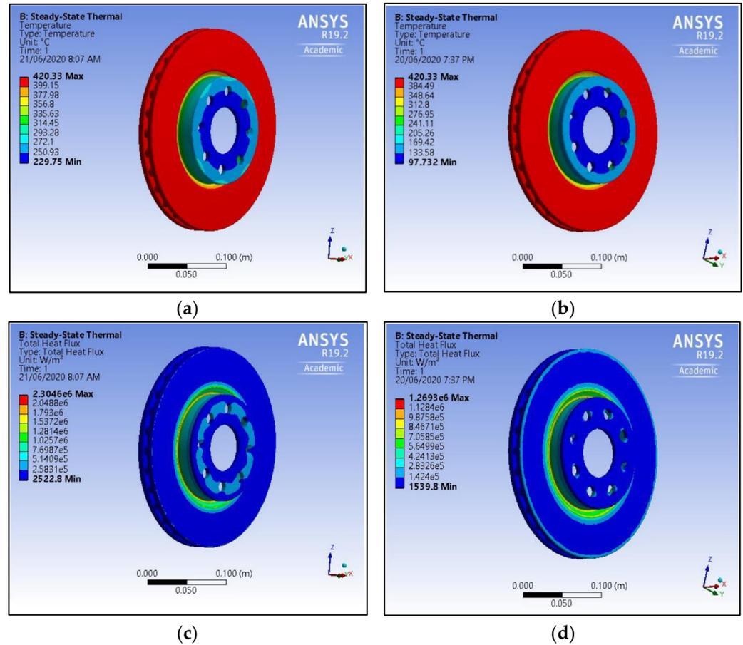
**Figure 5.** Thermal analysis of Al/SiC/Gr- and cast-iron-based brake rotors. (a) Temperature variation—Al6061/SiC/Gr, (b) Temperature variation—cast iron, (c) Total heat flux—Al6061/SiC/Gr, and (d) Total heat flux—cast iron.
