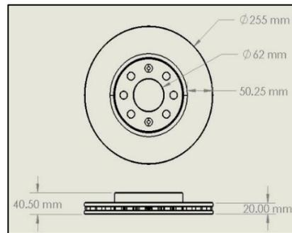
Figure 2. 2D view of brake disc.
