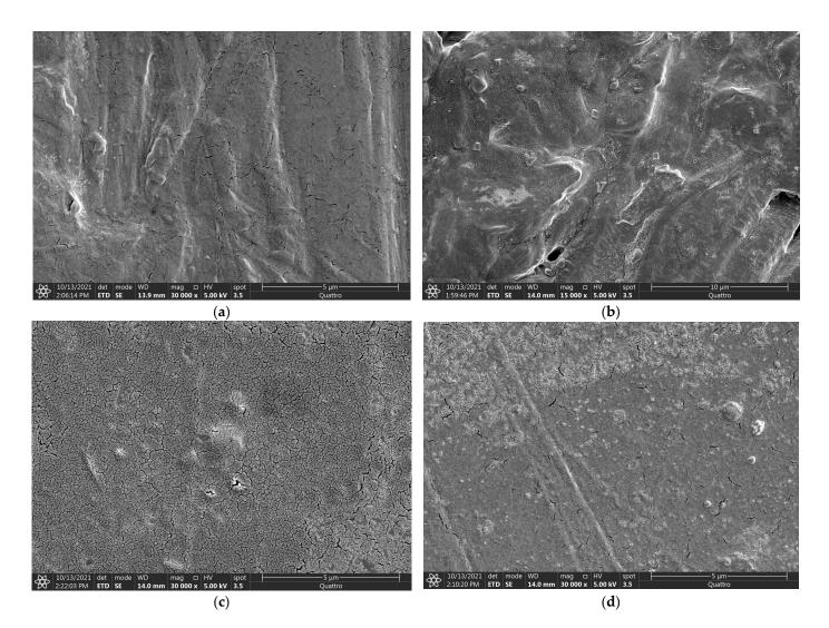
**Figure 3.** Scanning electron microscopy of wood composite samples at  $\times$  30,000 magnification for the (a) HDPE-control sample, (b) HDPE-18 wt. % wood sample, (c) PP-control sample, and (d) PP-18 wt. % wood sample.
