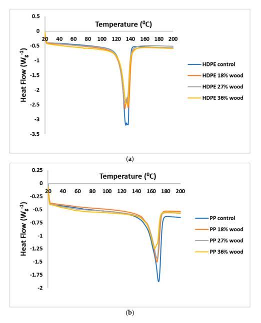
**Figure 2.** Differential scanning calorimetry of the (**a**) HDPE wood composite and (**b**) PP wood composite samples with different percentage weight of filler, shown as an overlay to illustrate the lack of any significant difference in the crystalline melt temperatures.
