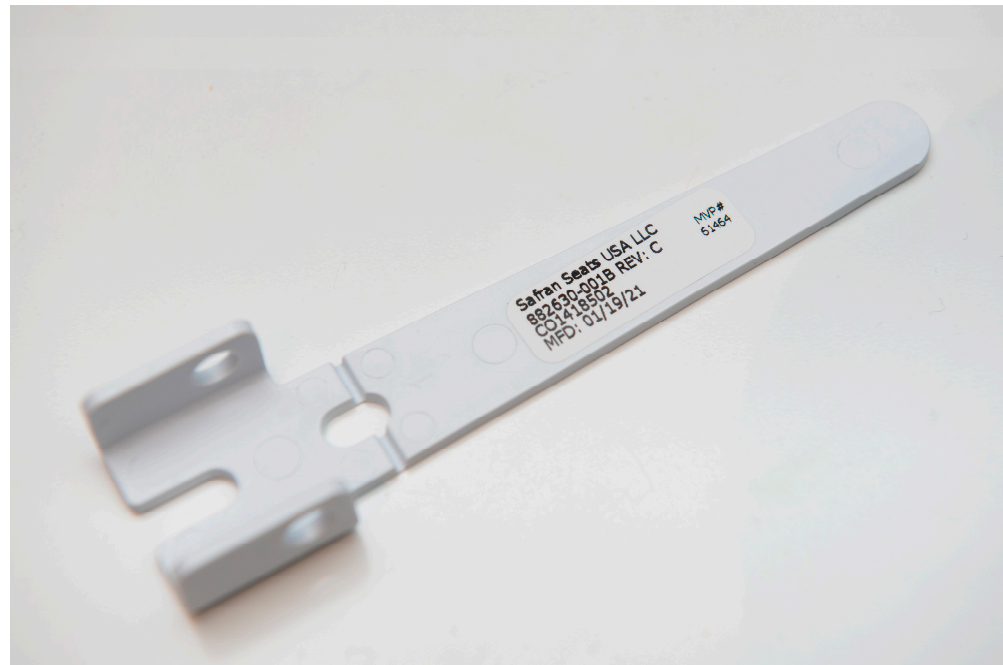
Figure 1. The studied aircraft part, namely, a finger pinch shroud from a Safran Seats US Z300 passenger seat.
