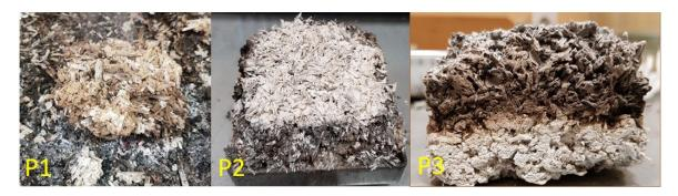
Figure 3. Samples after exposure to heat in the cone calorimeter test.
