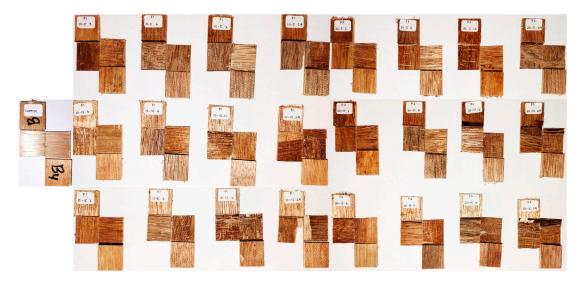
Figure 8. The wood failure images of plywood bonded with PVOH-tannin-hexamine-based adhesives.
