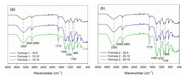
Figure 4. FTIR spectra of PVOH-tannin-hexamine-based adhesives. (a) Formula 1, (b) Formula 2.
