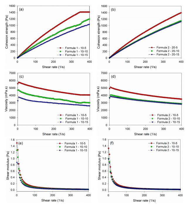
**Figure 3.** Flow behavior analysis of PVOH–tannin–hexamine-based adhesives. (**a**) Cohesion strength of Formula 1, (**b**) cohesion strength of Formula 2, (**c**) dynamic viscosity of Formula 1, (**d**) dynamic viscosity of Formula 2, (**e**) shear modulus of Formula 1, (**f**) shear modulus of Formula 2.
