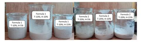
Figure 1. The PTH-based adhesive at different hexamine and tannin contents.
