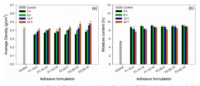
**Figure 5.** Physical properties of plywood bonded with PVOH–tannin–hexamine-based adhesives. (a) Average density, (b) moisture content.
