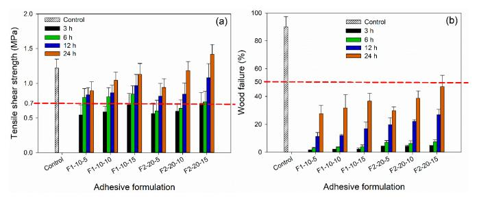
**Figure 7.** The bonding strength of plywood bonded with PVOH–tannin–hexamine-based adhesives. (a) Tensile shear strength, (b) wood failure.
