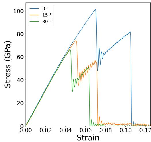
**Figure 9.** Tensile stress–strain curves under different angles of cracks for the composite structure formed by combining GE and IG (GE/IG).
