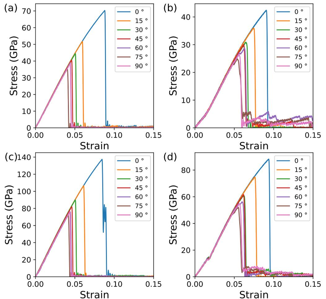
**Figure 8.** Tensile stress–strain curves under different angles of cracks: (a) monolayer graphene, (b) monolayer irida graphene, (c) bilayer graphene, (d) bilayer irida graphene.
