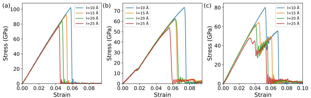
**Figure 6.** Tensile stress–strain curves of cracks of different lengths when the crack is 90° to the x-axis: (a) bilayer graphene (GE/GE), (b) double-layer irida graphene (IG/IG), (c) the composite structure formed by combining GE and IG (GE/IG).
