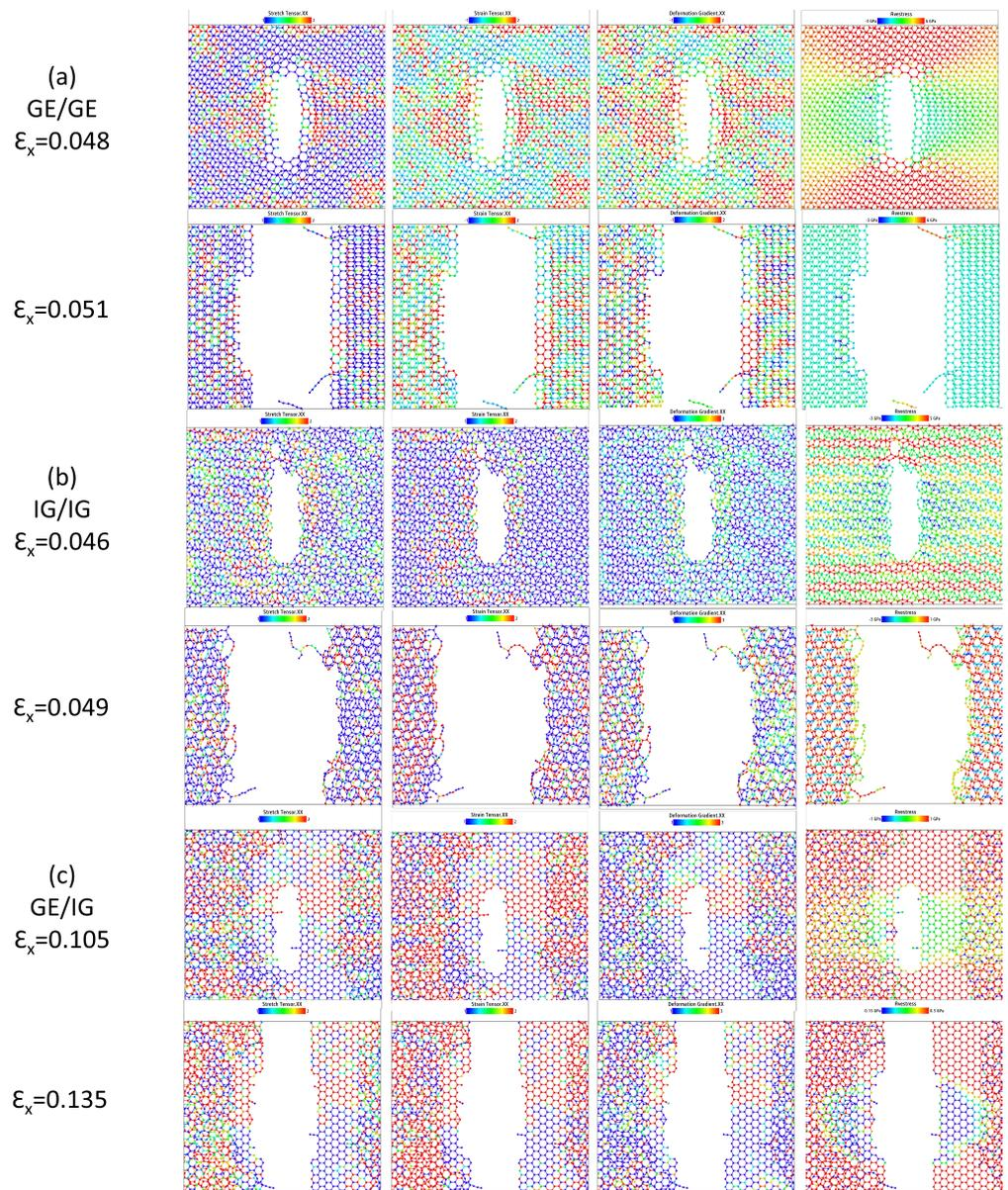
**Figure 7.** Fracture process of (a) GE/GE, (b) IG/IG, and (c) GE/IG.
