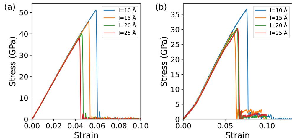
**Figure 5.** Tensile stress–strain curves under different numbers of atoms: (a) monolayer graphene (GE), (b) monolayer irida graphene (IG).
