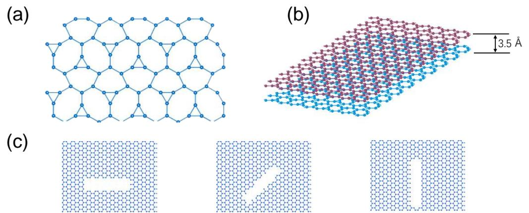
**Figure 1.** Schematic diagram of (a) the atomic structure of irida graphene, (b) bilayer irida graphene structure and (c) cracks, with angles of  $0^\circ$ ,  $45^\circ$ , and  $90^\circ$  to the tensile direction. The distance between layers is calculated using their relative coordinates.
