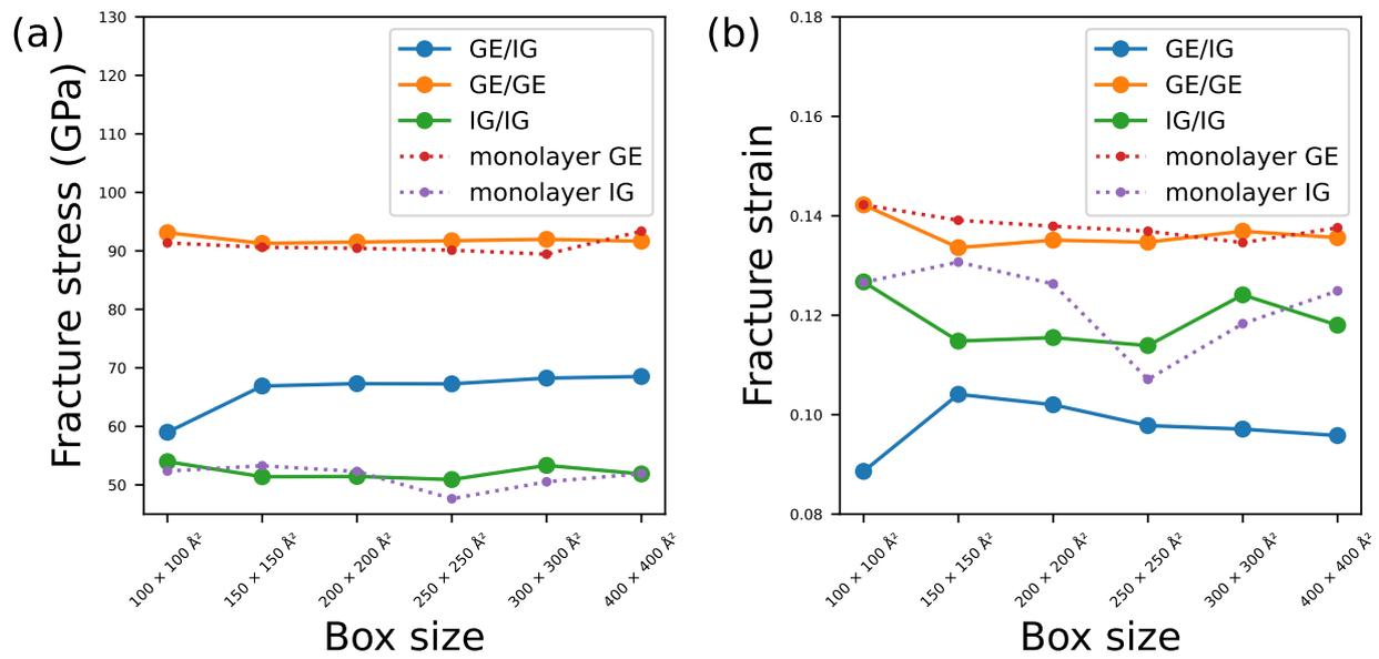
**Figure 4.** Fracture stress and strain at different box size: (a) relationship between fracture stress and box size, (b) relationship between fracture strain and box size.
