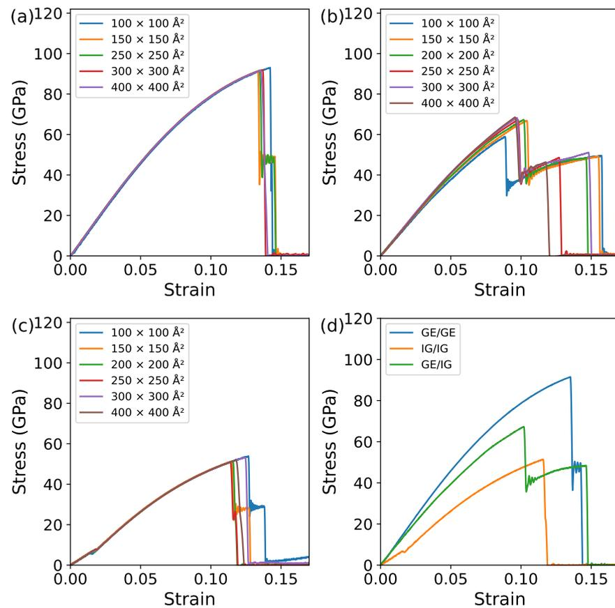
**Figure 3.** Tensile stress–strain curves under different atoms: (a) double-layer graphene (GE/GE), (b) double-layer irida graphene (IG/IG), (c) the combination of one layer of graphene and one layer of iridium graphene structure (GE/IG), (d) comparison of stress–strain curves of three structures with box size of  $200 \times 200 \text{ \AA}^2$ .
