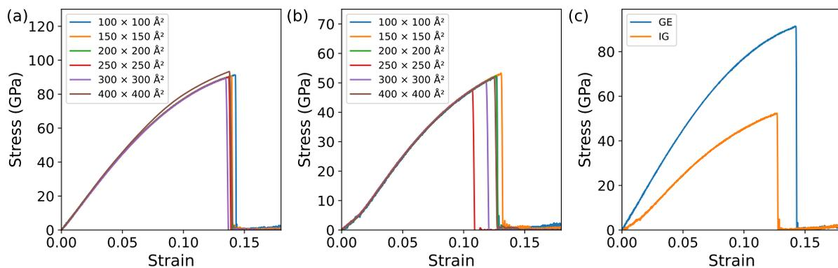
**Figure 2.** Tensile stress–strain curves under different numbers of atoms: (a) monolayer graphene (GE), (b) monolayer irida graphene (IG), (c) comparison of stress–strain curves of two structures with box size of  $200 \times 200 \text{ \AA}^2$ .
