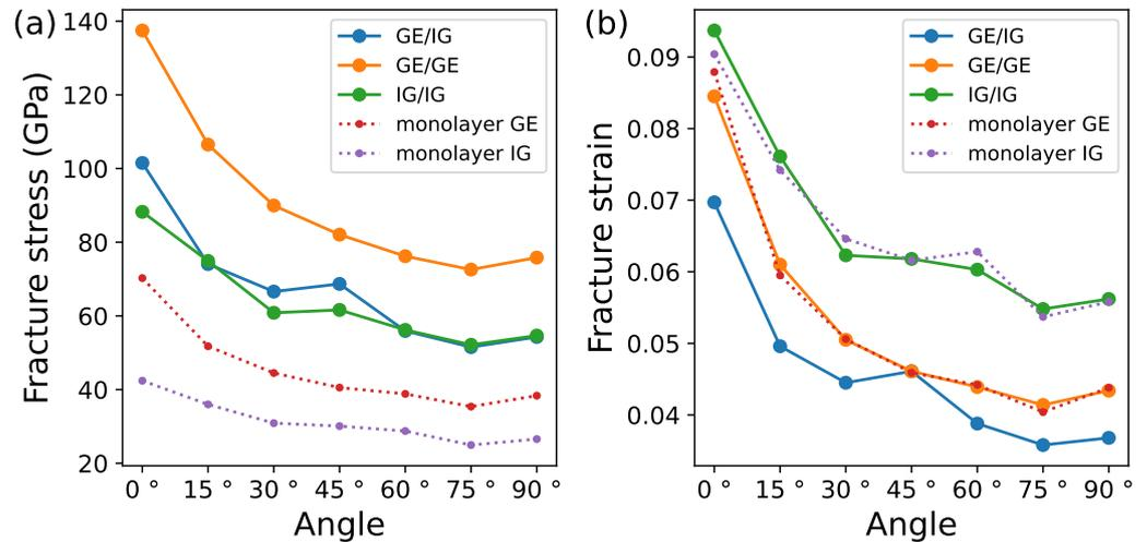
**Figure 10.** Fracture stress and strain at different crack angles: (a) relationship between fracture stress and crack angle, (b) relationship between fracture strain and crack angle.
