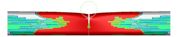
Transverse (matrix) compressive failure—MAT54 history variable 4:
