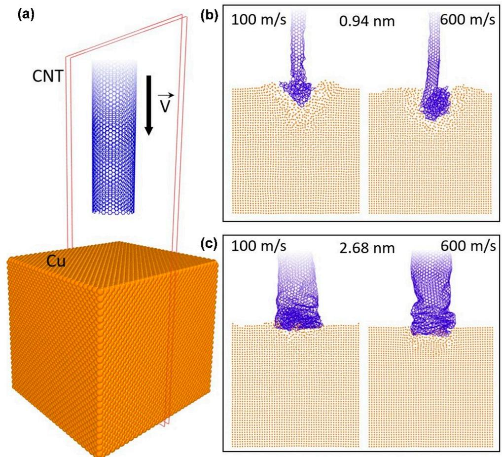
**Figure 4.** Schematic presentation of the molecular dynamic simulation. (a) Presentation of the CNT deposition into the copper substrate. (b) Interaction of CNT with a diameter of 0.94 nm with copper substrate at the acceleration rate of 100 and 600 m/s. (c) Interaction of CNT with a diameter of 2.68 nm with copper substrate at the acceleration rate of 100 and 600 m/s.
