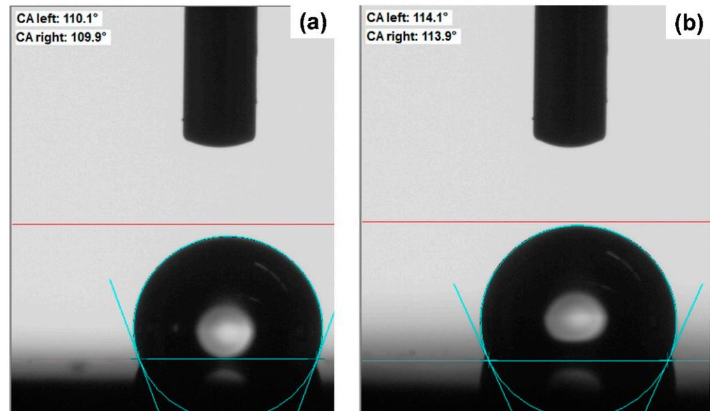
**Figure 3.** The CA of (a) original copper and (b) CNTs-deposited surface.
