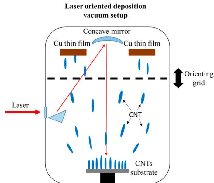
**Figure 1.** The laser-oriented deposition scheme used for the Cu-surface modification.
