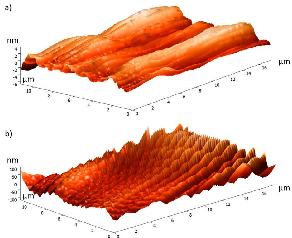
**Figure 5.** AFM-3D images of pure Cu (a) and Cu structured with the CNTs (b).
