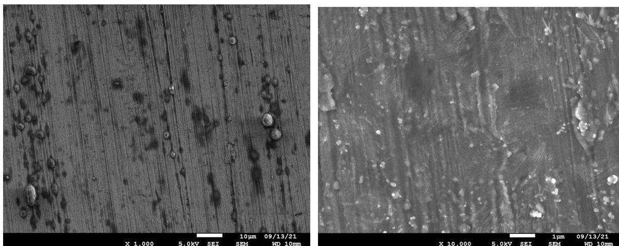
**Figure 6.** SEM images of the pure Cu (left figure) and Cu structured with CNTs (right figure).
