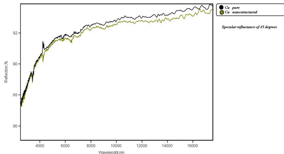
**Figure 2.** Reflectance spectra of the CNTs-deposited surface and the original copper.
