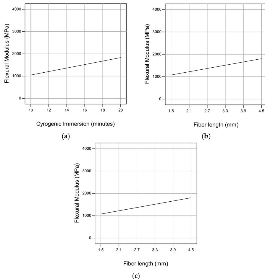
**Figure 4.** Effect of the individual factors on flexural modulus: (a) effect of cryogenic treatment; (b) effect of fiber length; (c) effect of fiber orientation.
