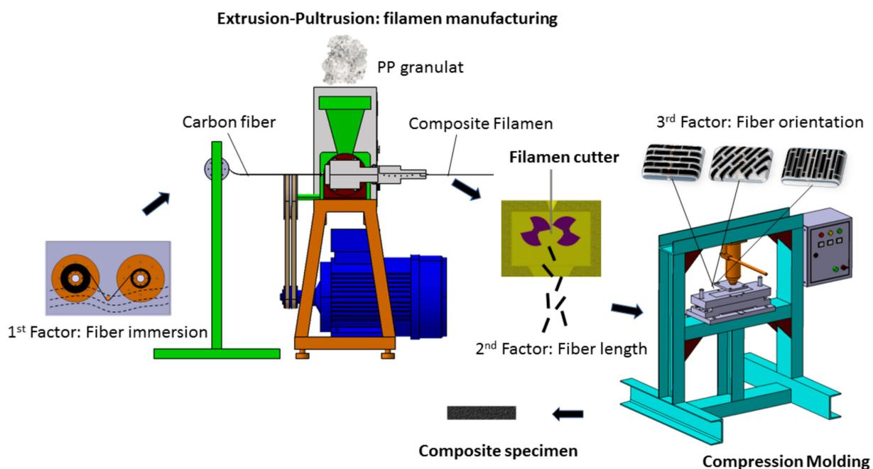
**Figure 2.** Preparation of composite specimen involving three factors: fiber immersion, fiber length, and fiber orientation.
