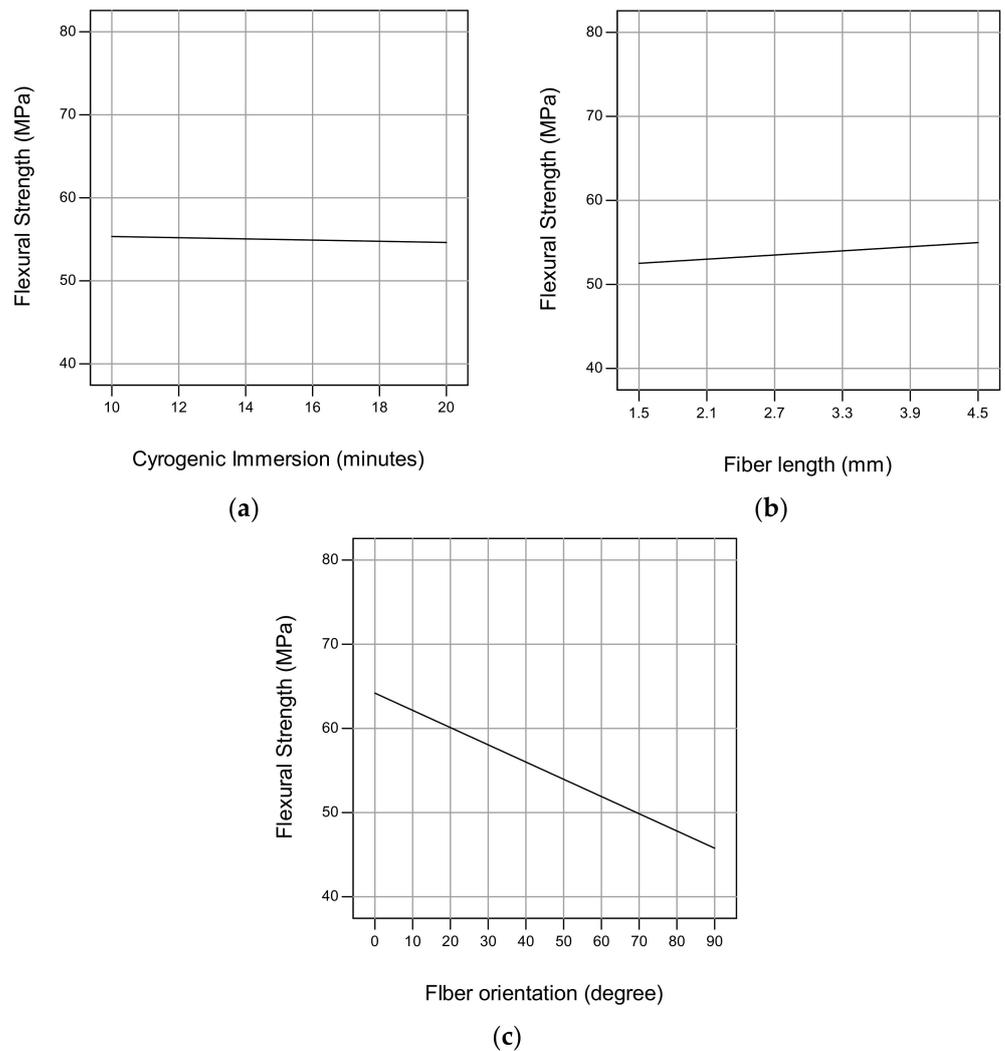
**Figure 3.** Effect of the individual factors on flexural strength: (a) effect of cryogenic treatment; (b) effect of fiber length; (c) effect of fiber orientation.
