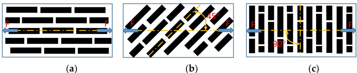
**Figure 1.** Fiber orientation with the respect to load direction: (a) 0 $^{\circ}$ ; (b) 45 $^{\circ}$ ; (c) 90 $^{\circ}$ .
