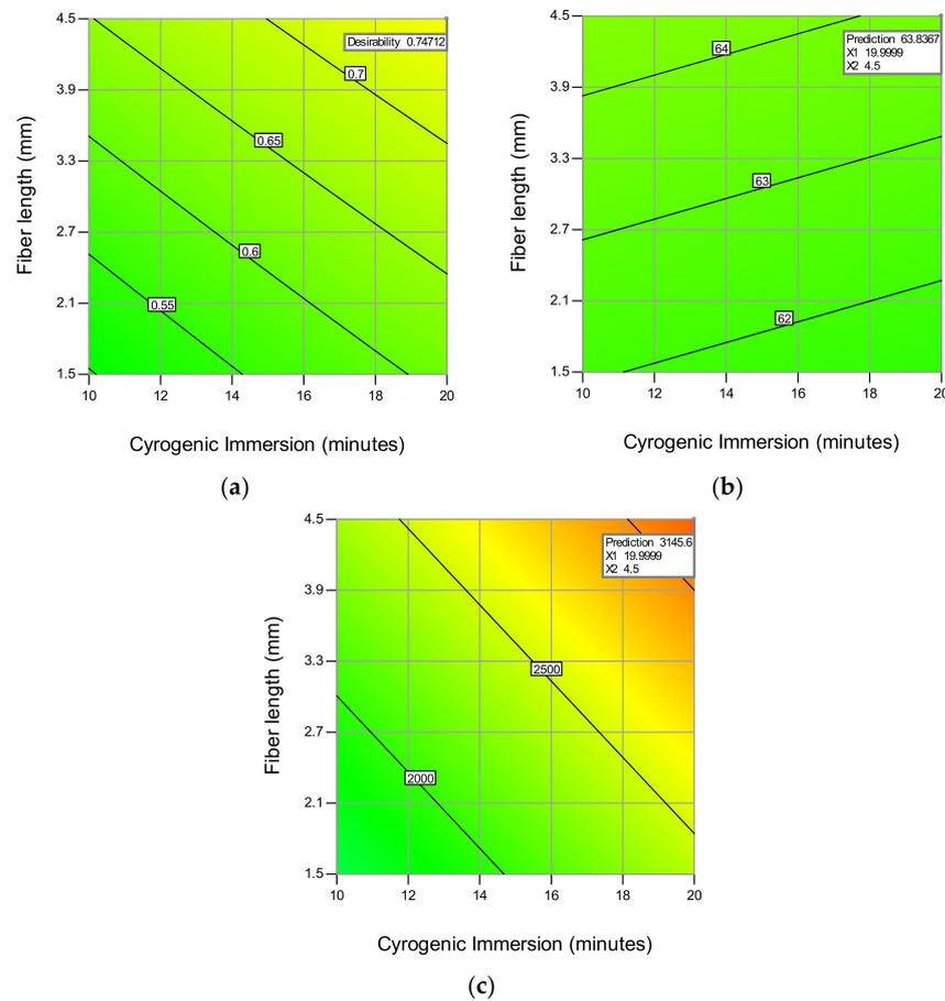
**Figure 5.** Optimized responses defined by desirability function: (a) desirability; (b) optimized flexural strength; (c) optimized flexural modulus.
