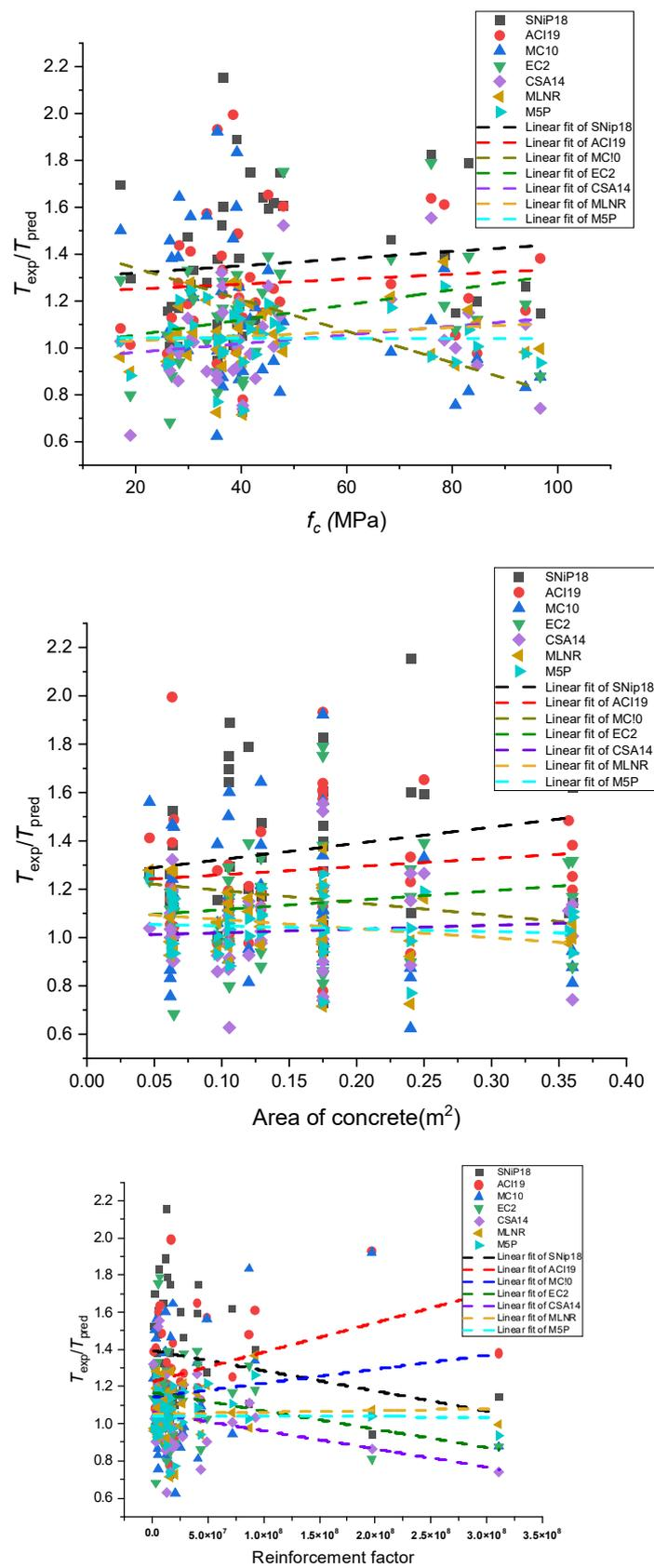
Figure 5. Relationship between the variables and the ratio of experimental to predicted torsional strength.
