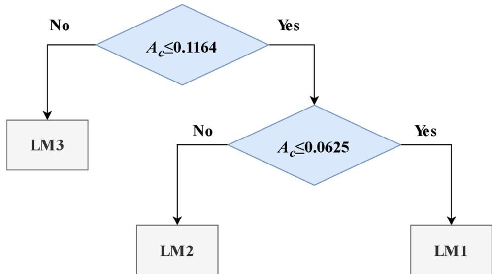
Figure 3. M5P algorithm-based tree developed to estimate the torsional resistance of RC beams.
