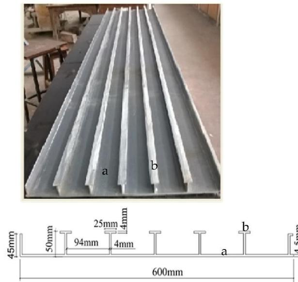
Figure 1. FRP-SIP used in the experiments.
