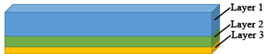
Figure 10. Three-dimensional (3D)-printed composite bearers with multi-layers.
