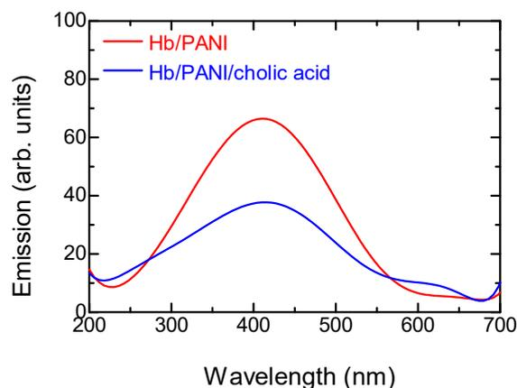
**Figure 5.** Photoluminescence (PL) spectra of Hb/PANI and Hb/PANI/cholic acid in luminol solution.
