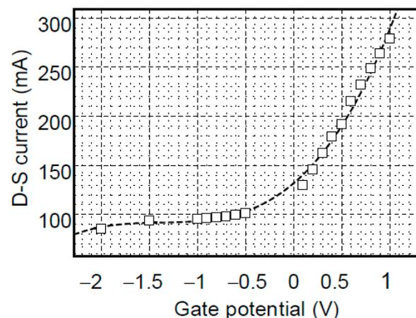
Figure 7. Change in drain–source current with gate potential for Hb/PANI as an electrochemical-field effect-type transistor (e-FET).
