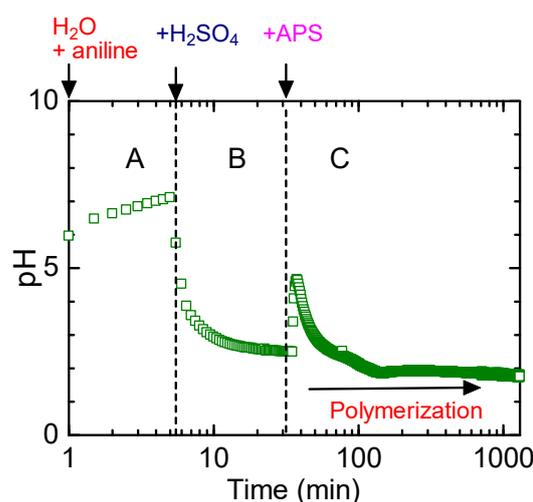
**Figure 1.** Change in pH during polymerization. Change in pH after the addition of aniline (A). Change in pH after the addition of sulfuric acid (B). Change in pH after the addition of ammonium peroxodisulfate (APS) (C).
