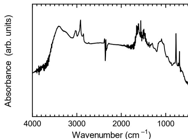
**Figure 3.** Fourier transform infrared (FT-IR) absorption spectra of Hb/PANI/cholic acid.
