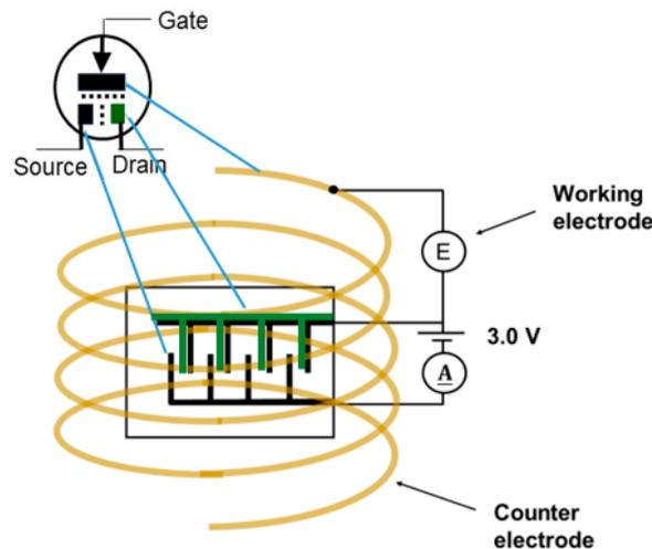
Figure 6. Hb/PANI-based electrochemical transistor.
