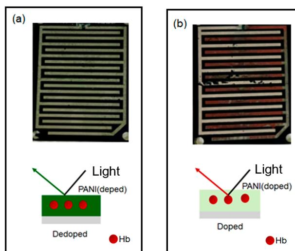
**Figure 8.** The appearance of Hb/PANI deposited on interdigitated array electrodes for an electrochemical transistor and the possible mechanism of the color change upon doping–dedoping. (a) Doping. (b) Dedoping.
