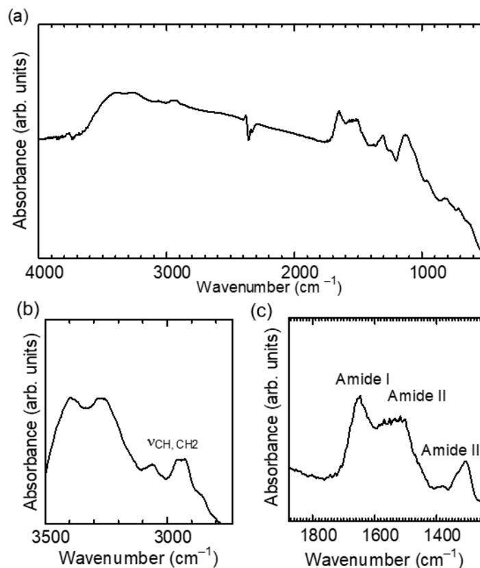
**Figure 2.** (a) Fourier transform infrared (FT-IR) absorption spectra of Hb/PANI. (b,c) Magnification of the IR absorption spectra of Hb/PANI. Hb: hemoglobin.
