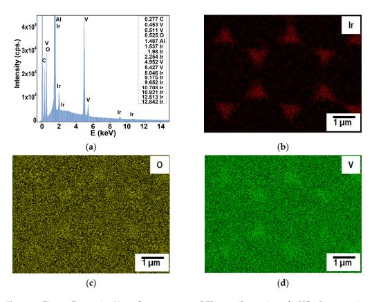
**Figure 4.** Energy Dispersive X-ray Spectroscopy and Elemental mapping of a VO<sub>2</sub>–Ir composite. The thickness of VO<sub>2</sub> 200 nm and the "a" parameter of Ir microtriangles is equal to 0.70  $\mu$ m (a) EDS elemental analyses of the composite; (b) Elemental map of Ir microtriangles; (c) Elemental map of Oxygen; (d) Elemental map of Vanadium.
