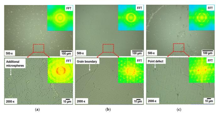
**Figure 2.** Temperature dependence of the 2D arrangement of polystyrene microspheres (P-spheres) with a 3-micrometer diameter on an  $Al_2O_3$ -c substrate: (a) P-spheres deposited at 20 °C using Langmuir–Blodgett colloidal lithography (LB); (b) P-spheres deposited at 25 °C using LB; (c) P-spheres deposited at 30 °C using LB. The insert images in Figure 2 represent the Fast Fourier transform (FFT) of the underlaying optical images of the LB results.
