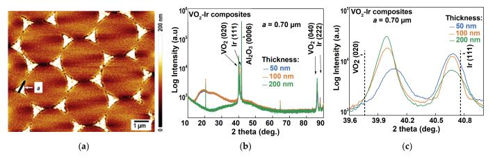
Figure 3.  $VO_2$ –Ir microtriangles composite's morphological and structural characteristics: (a) AFM image; (b)  $\theta$ -2 $\theta$  XRD patterns; (c) Zoom on a part of (b) XRD patterns from 39.6° to 41°  $\theta$ -2 $\theta$  XRD patterns of the composite. The thickness of the Iridium triangles within the composite is fixed to 50 nm, while the  $VO_2$  thickness is 50, 100 and 200 nm. The dotted lines in image (c) correspond to the theoretical position of  $VO_2$  and Iridium.
