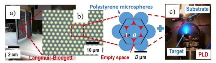
**Figure 1.** VO<sub>2</sub>–Ir microtriangles composites' manufacturing pathway. (a) Photography of a perpendicular substrate covering by polystyrene spheres (P-spheres). (b) Schematic of spheres (P-spheres) compact arrangement. (c) Photography of a pulsed laser deposition process.
