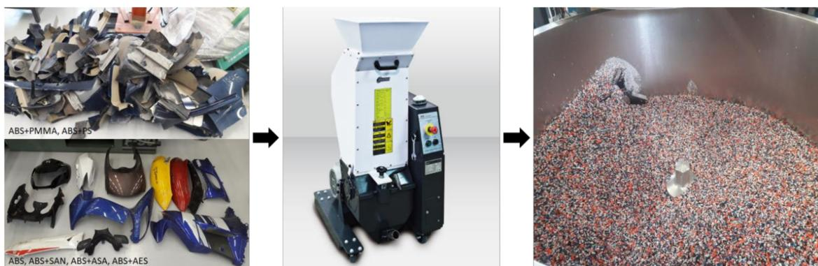
**Figure 7.** Illustration of the crushing process for the waste automotive components.
