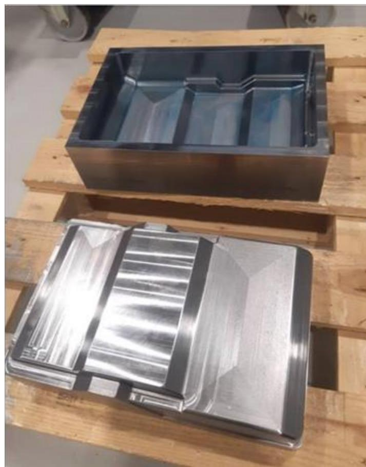
**Figure 5.** Compressing molding tool manufacturing to produce natural fiber polymer composite (NFPC) components.
