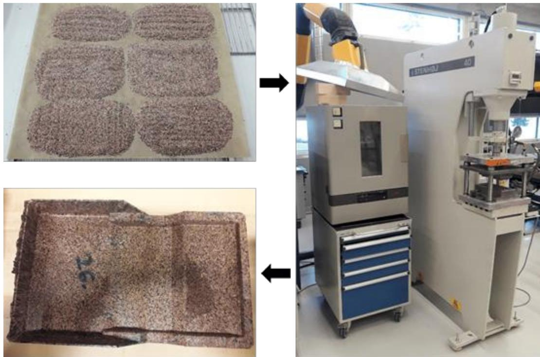
**Figure 8.** Compression molding setup and the production of the new automotive part.
