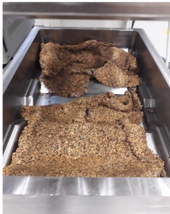
**Figure 10.** Evenly spread material placement, especially on the edges of the tool, provides optimal results.
