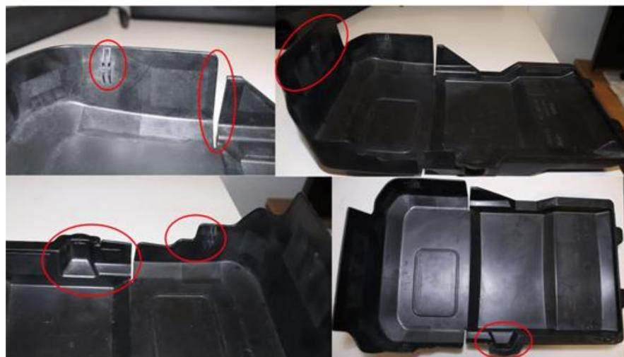
Figure 3. Complex features in the existing component.
