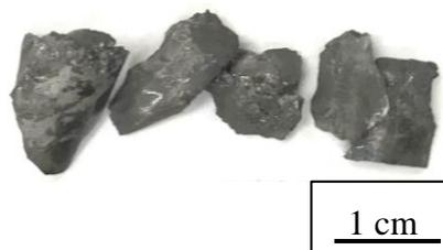
**Figure 8.** Fragments of the fractured steel core retrieved from Armor 2 (PP) following testing.
